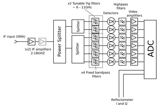
Figure 4: The IF section contains six parallel filter channels, two of which are tunable YIG filters of 200MHz bandwidth. The tunable filters provide flexibility in radial coverage and may extend the region of the plasma where a match to the reflectometer position may be found.
