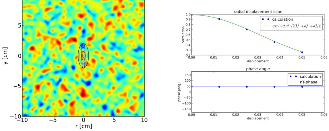
Figure 2: (a) An example of the spatial point spread functions taken for the reflectometer and CECE. The CECE radial width is taken to be that of the relativistic broadening at 1keV. (b) Maximum coherence and phase angle as a function of radial displacement. Notice that while the measured coherence is reduced, the phase angle is unaffected in this case.
