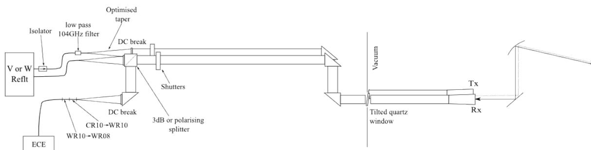
Figure 5: The waveguide transmission line for the CECE radiometer/reflectometer pair. Either a 3dB or polarising splitter can be interchanged to allow coupling to either X or O mode reflectometers.
