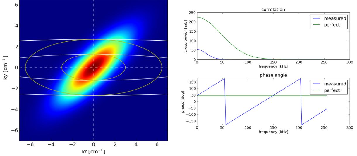
Figure 3: (a) The  $k$ -space distribution showing an exaggerated tilt. (b) The correlation analysis for the tilted  $k$ -space distribution, for a single displacement. One can see that the asymmetry around  $k_r = 0$  results in an effective time delay, leading to a phase dispersion in the measurement.
