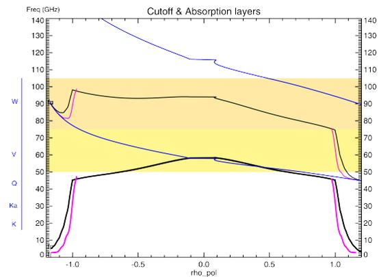
Figure 1: The cutoffs and resonances for a typical 2.5T ASDEX Upgrade discharge. One may select a frequency for either O or X mode reflectometers to be coincident in radius with a 2nd harmonic X mode CECE channel.
