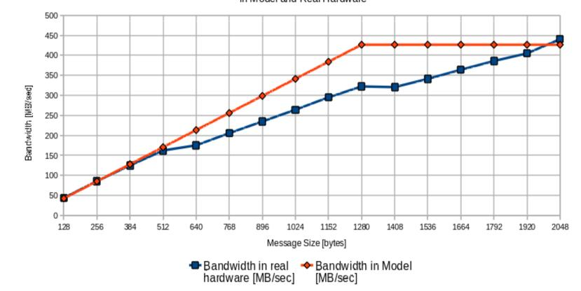
Bandwidth Measurements in Model and Real Hardware
