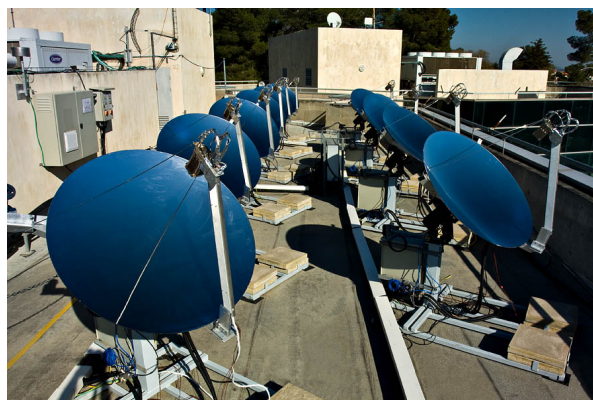
Figure 1: Experimental field of concentrating PV/thermal collectors.
