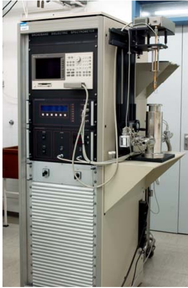
Dielectric spectrometer novocontrol (high frequency device)
