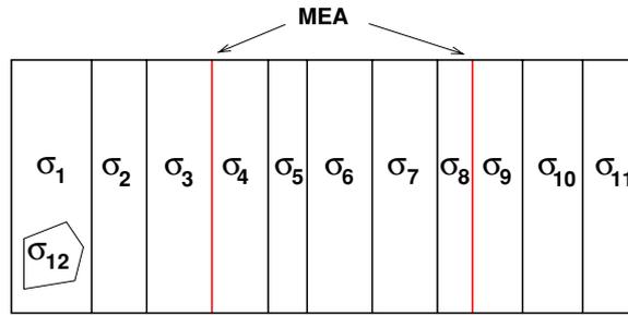
**Figure 2.** Schematic representation of a fuel cell stack (with 2 MEAs only) build up from 12 connected areas  $G_i$  of materials with different conductivities. One possible permutation is  $p(1) = 12, p(2) = 1, p(3) = 2, p(4) = 3$ , etc.  $G_b$  fulfills all requirements of definition 1.
