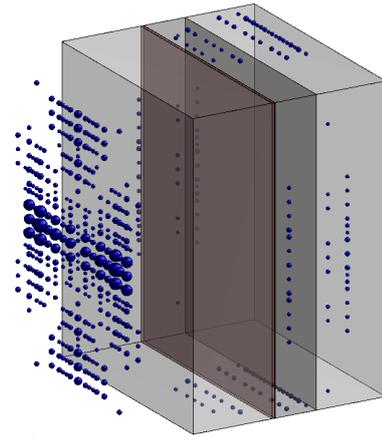
*FIG. 1: Reduced measuring point distribution for the magnetotomography of a single fuel cell with a cross section of  $138 \text{ mm} \times 178 \text{ mm}$ . The size of the spheres denotes the importance of the measuring points. Their number, originally 6702, is reduced to 498. It is obvious, that the most important ones are located on the front side of the fuel cell.*
