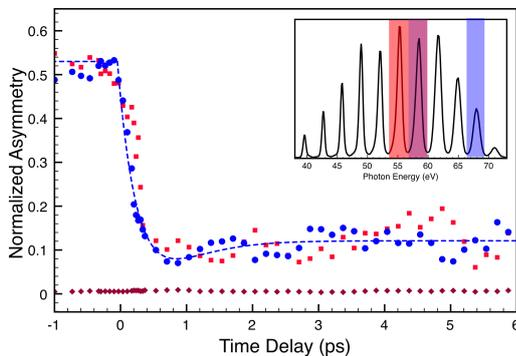
FIG. 3: Time-resolved measurement of the femtosecond laser-pulse induced demagnetization of the Permalloy film by high-harmonic photons around the Ni (blue circle), Fe (red square)  $M$  edge, and off-resonance (diamond). The dashed line corresponds to a fit of the expected response [3].
