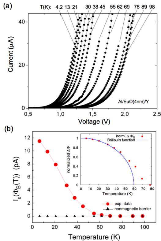
FIG. 2: (a)  $I-V(T)$  plot of an Al/EuO(4 nm)/Y spin filter tunnel junction at positive bias. (b) Saturation current  $I_0(\Phi_{\uparrow(\downarrow)}(T))$  as a function of  $T$ , shown together with the result for a nonmagnetic barrier. The inset shows the normalized change in effective barrier height  $\Delta\Phi(T)$  fitted to a Brillouin function with  $S = 7/2$ .
