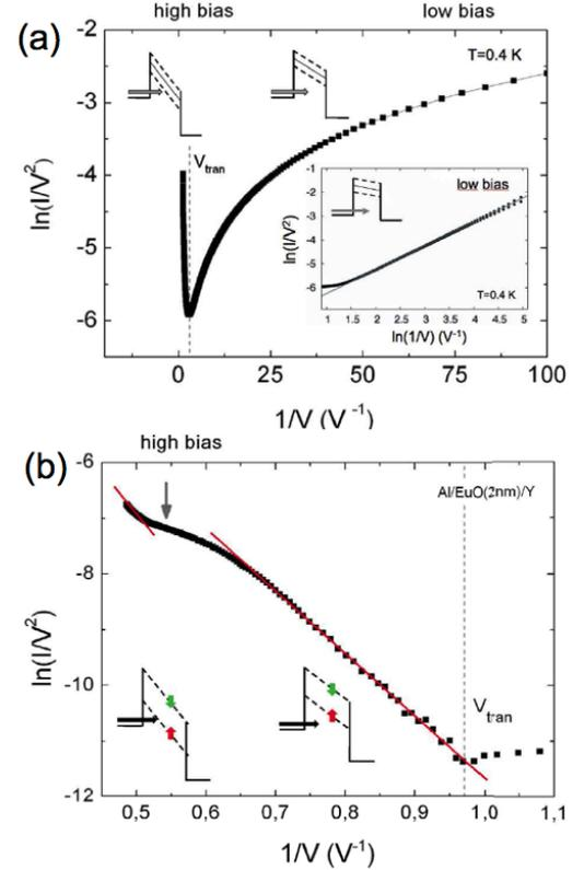
FIG. 1: (a)  $\ln(I/V^2)$ - $1/V$  plot of an Al/EuO(4 nm)/Y junction at  $T=0.4$  K. The dotted line denotes the transition voltage at which the transport mechanism changes from DT to FN tunneling. (b)  $\ln(I/V^2)$ - $1/V$  plot for the high bias region of an Al/EuO(2 nm)/Y junction. Two onsets of linear decaying slopes are observable, separated by a crossover region.
