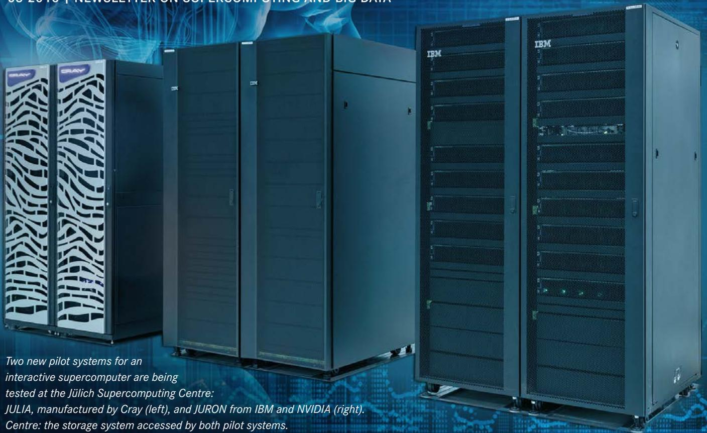
*Two new pilot systems for an interactive supercomputer are being tested at the Jülich Supercomputing Centre: JULIA, manufactured by Cray (left), and JURON from IBM and NVIDIA (right). Centre: the storage system accessed by both pilot systems.*
