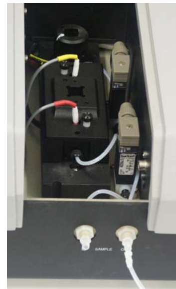
Figure 2: Interior of the Zetasizer with fully mounted capillary M3 cell
