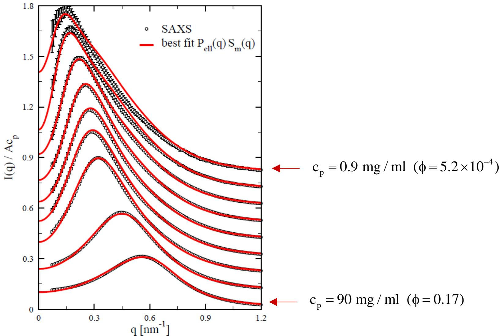
Interaction parameters fully determined from SAXS fit
