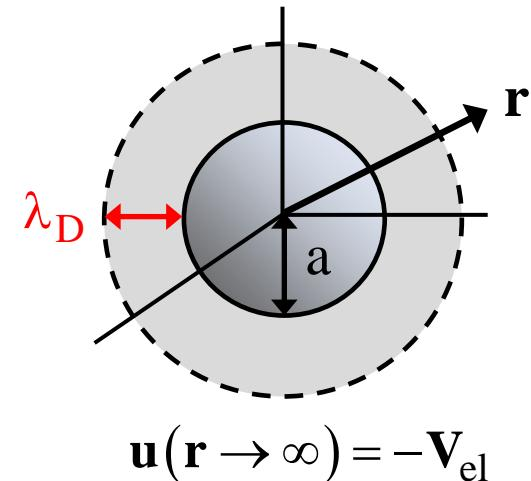
$$\mathbf{F}^{\text{h}} = 6\pi\eta_0 a \left[ 1 + \frac{a^2}{6} \Delta \right] \mathbf{u}_{\text{in}}(\mathbf{r} = \mathbf{0}) \quad \begin{aligned} &\text{hyd. drag force on stationary neutral sphere with stick BC} \\ &\text{in incident flow field created by sources outside the sphere} \end{aligned}$$
