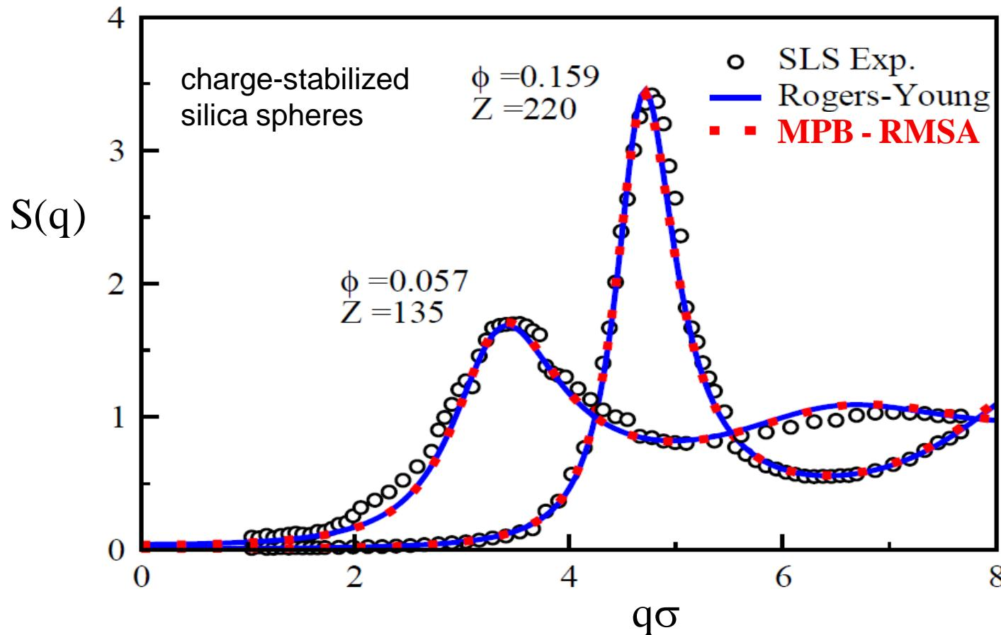
**MPB - RMSA:** scheme close to experiment, simulation & RY scheme
