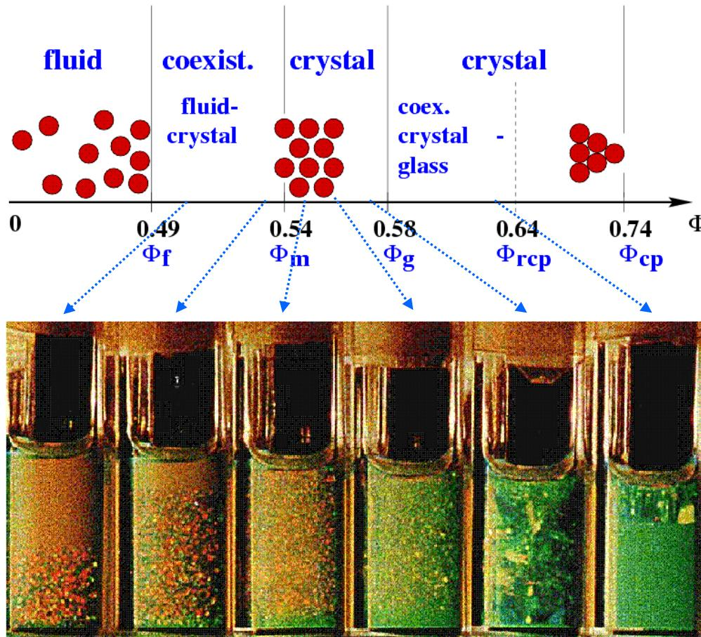
$$\phi = \frac{Nv_{\text{sphere}}}{V_{\text{system}}} = \frac{4\pi}{3} n a^3$$
