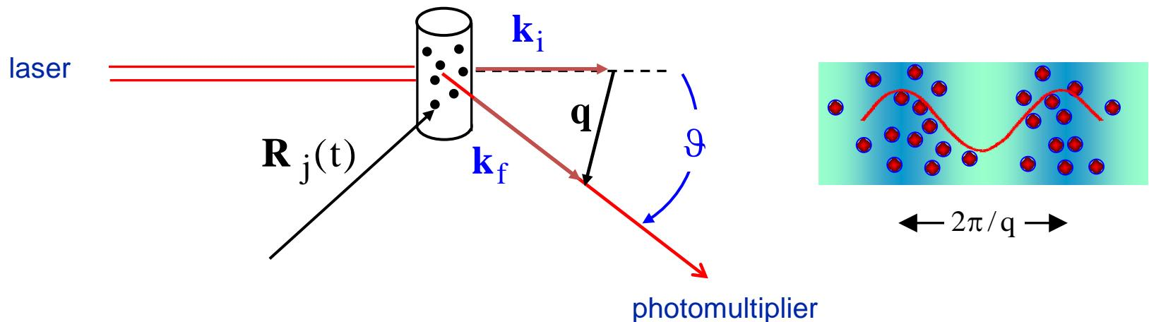
$$I(q) \propto \langle N \rangle P(q) S(q) \quad : \text{for single and quasi-elastic scattering} \quad q = \frac{4\pi}{\lambda} \sin \left[ \frac{\theta}{2} \right]$$
