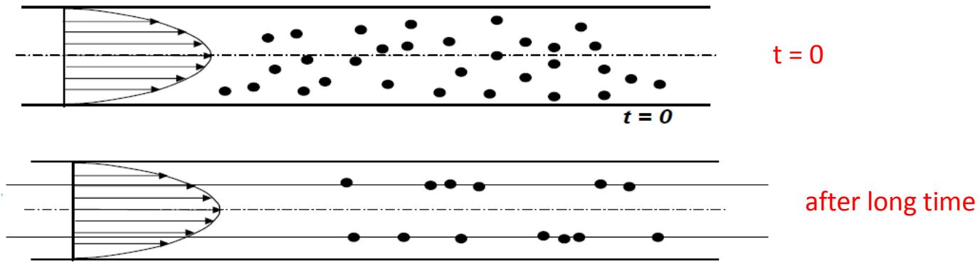
Lift force drives particles towards ring at  $r / R \approx 0.6$  (inertia effect)
