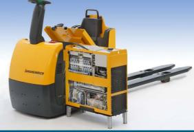
**Power Units for Light Traction and Uninterruptable Power Supply Applications**
