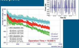
"Jülich, 10 February 2012 – Ten thousand hours in operation: Scientists from Forschungszentrum Jülich set up this record with a hybrid system based on direct methanol fuel cells (DMFCs).
