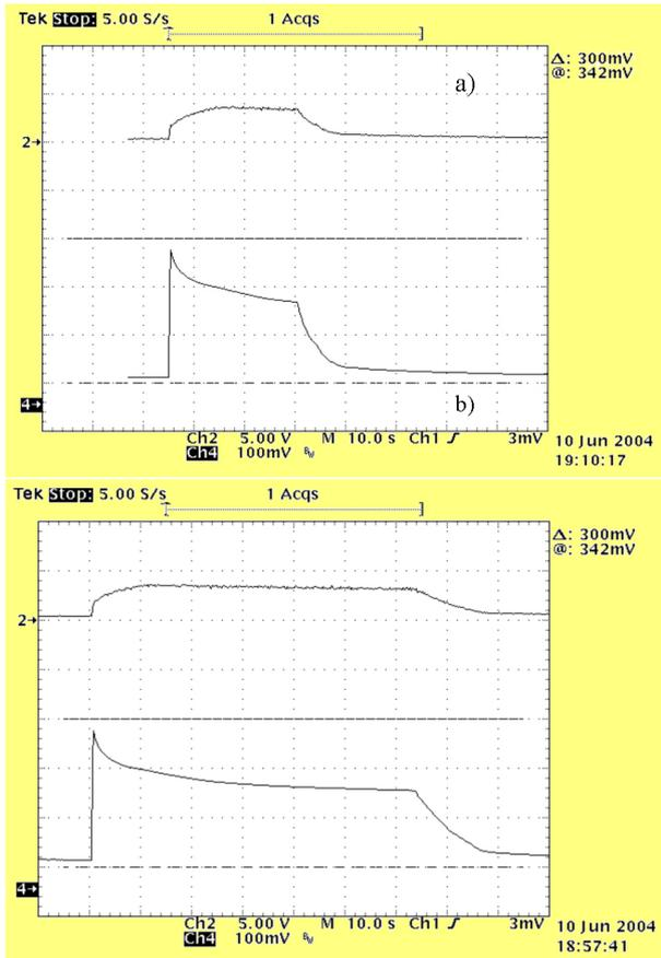
Fig. 37: Proton beam current (lower curves) and  $H^0$  count rate (upper curves) versus time: a) Shaker is off or non-resonant excitation, One division corresponds to 1 mA beam current. b) Excitation with the resonant frequency of 114 kHz.. One division corresponds to 1 mA beam current.
