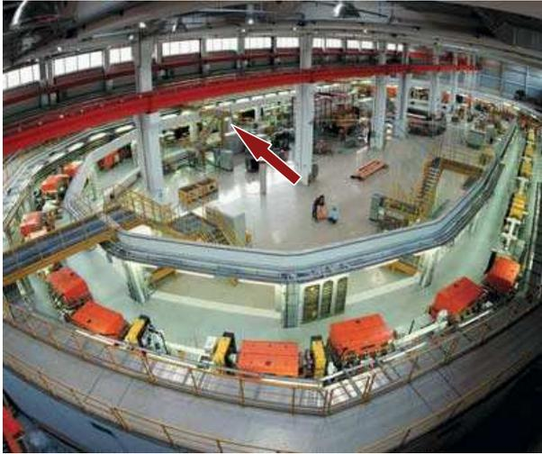
Fig. 11: The COSY accelerator hall. The arrow indicates the future position of WASA in one of the straight sections of COSY.
