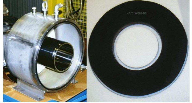
Fig. 43: Barrier Bucket cavity (left), magnetic alloy core for acceleration cavity (VitroPerm®, right)
