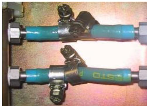
**Fig. 3:** Defect hoses, very often with little holes or porous.
