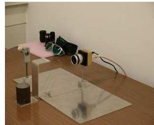
Fig.2 Photograph of the system used to determine the thickness a hair.
