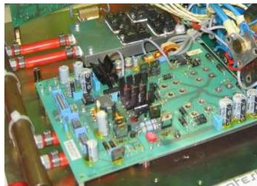
**Fig. 4:** Blue tubes in figure 3 replaced by more durable ones (red).
