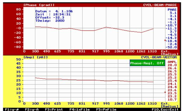
Fig. 2: Beam transmission through the cyclotron as the demonstration for the improved situation in 2006.
