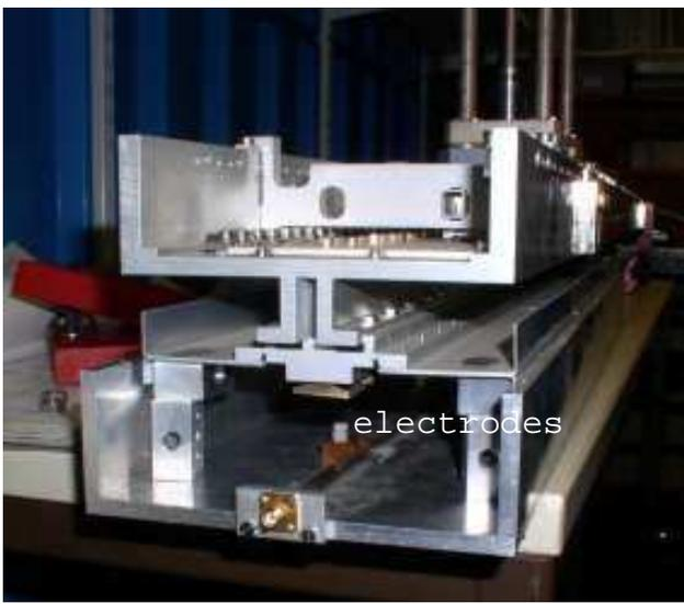
**Fig. 3:** COSY cooling structure and test bench. The length in the beam direction reaches about 0.25m (8 electrodes).
