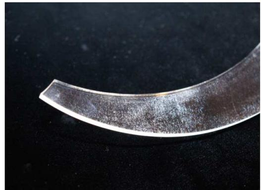
Fig. 2: Unwrapped scintillator of the FTH. Light is reflected from the microcracks.
