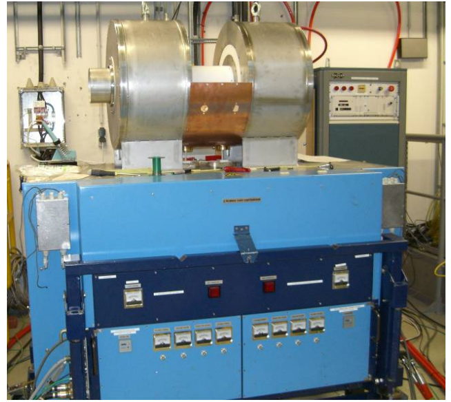
Fig. 2: Prototype of HESR accelerating cavity installed on top of the former COSY tube amplifier.
