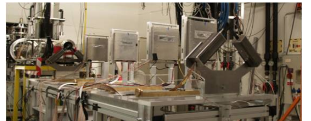
Fig. 49: Silicon strip tracking station for beam test at COSY.
