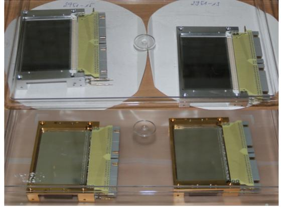
Fig. 37: The fabricated Si with Aluminum holder (upper) and Ge with Copper frame (lower) detector of recoil arm.
