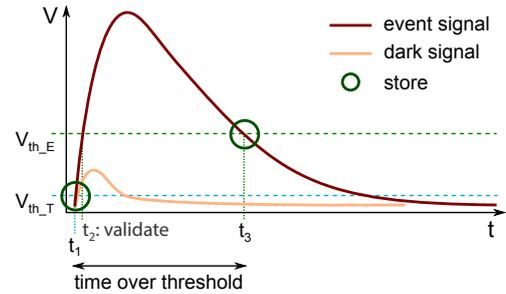
Fig. 48: A simplified signal after the pre-amplifier. Two discriminator levels deliver four points in time,  $t_1$  and  $t_3$  are stored in the default operation mode for the time of arrival and the time over threshold. Only if the signal exceed  $V_{\text{th},E}$  it is processed.
