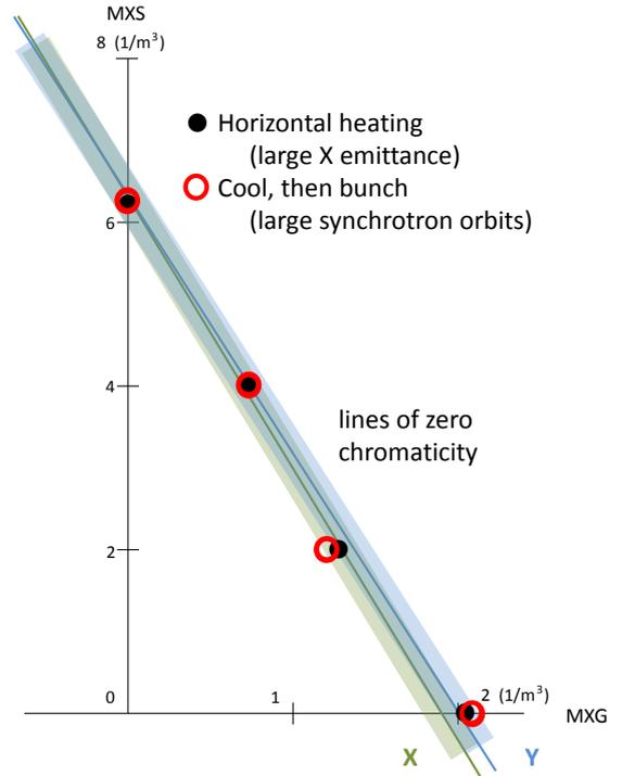
Fig. 34: On the plane of MXS and MXG sextupole values, the two bands indicate the error margin for locating the places where the X or Y chromaticity is zero (with MXL set to  $-0.2 / m^{-3}$ ). Scans of the polarization lifetime using two different beam setups (horizontally wide and longitudinally extended) gave values where the polarization lifetime went through a maximum, which is shown here by either a black dot or a red ring.
