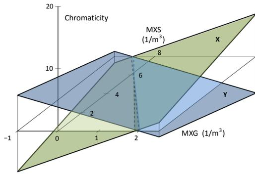
Fig. 33: The two planes in this projection drawing show the values of the X and Y chromaticities as functions of the settings of the fields in the MXG and MXS sextupole families. The shading of the two planes is meant to illustrate where the chromaticity is positive or negative (or visible around the edge of the zero chromaticity plane). Dashed lines show where these planes cross zero chromaticity.
