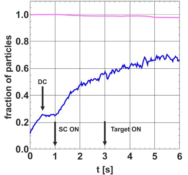
Fig. 41: Fraction of ions with relative momentum spread within  $|\Delta p/p| \leq 5 \cdot 10^{-5}$  (blue) and  $3 \cdot (\Delta p/p)_{inj}$  at injection (magenta) versus time. At 500 ms (DC) the final barrier position is reached. The beam is now nearly a DC beam. Stochastic TOF cooling is switched ON at  $t = 1$  s (SC ON). The target is inserted at  $t = 3$  s (Target ON).
