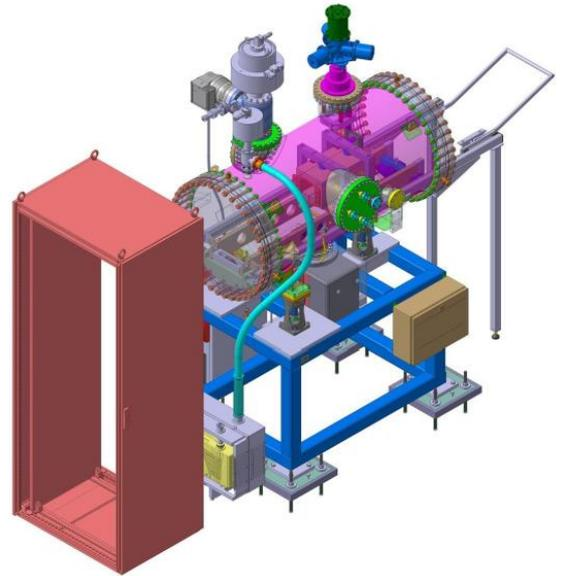
Fig. 40: Test tank for injection kicker magnets.
