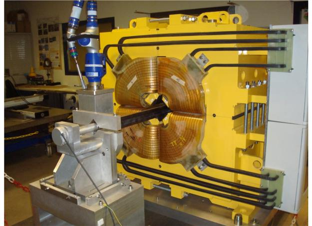
Fig. 38: Quadrupole magnet on measuring bench.
