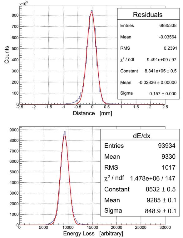
Fig. 51: Results of the beam tests for the FADC-based readout. Upper: Residual distribution of reconstructed tracks for 1.3 GeV/c proton beam. Lower: Specific energy-loss distribution (dE/dx) for the same proton beam momentum and after truncating the 20 % track hits with highest dE/dx.
