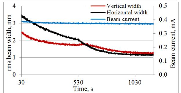
Fig. 25: Evolution of the beam width and beam current during transverse stochastic (first half of the machine cycle) and electron cooling with 320 mA (second half).
