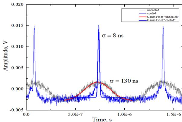
Fig. 27: Electron cooling of bunched proton beam at 1670 MeV. Shown are the bunch shapes for the cooled and uncooled proton beam as reported by the bunch phase monitor.
