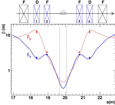
Fig. 18: Model calculation of the  $\beta$ -functions at the PAX-TP and measured values of  $\beta_x$  and  $\beta_y$  at the magnet positions. In blue the four new PAX quadrupole magnets are indicated. Magnet 1 and 4 form the defocusing (D) pair (PAX1), while magnets 2 and 3 the focusing (F) pair (PAX2). Each pair is operated with a single power supply. In addition the storage cell and the beam direction are shown.
