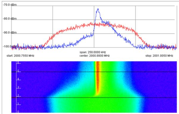
Fig. 26: Longitudinal electron cooling of proton beam at 1670 MeV. A pickup of the stochastic cooling system was used to measure the Schottky spectra. Only a part of the machine cycle is shown. Transverse stochastic cooling was active until  $t = 2$  min, after that electron cooling was turned on. In the upper plot the red curve corresponds to the longitudinally uncooled beam while the blue one shows the spectrum of the cooled beam.
