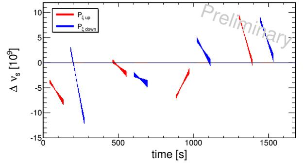
Fig. 29: Walk of the spin tune during eight consecutive cycles with alternating initial vector polarization. The third cycle is depicted in Fig. 28 as well. Cycles with unpolarized beam that followed the down state (blue) are not shown.
