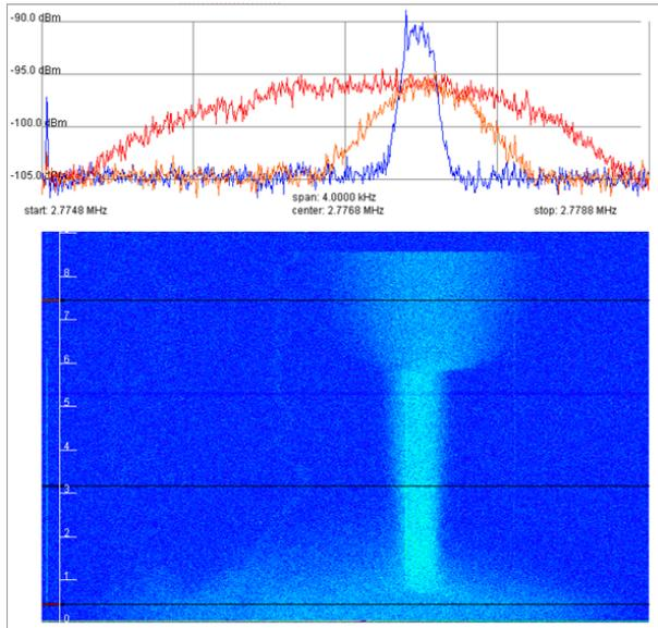
Fig. 22: Evolution of the longitudinal Schottky spectra. The 200 mA electron beam was turned on at  $t = 30$  s and turned off at  $t = 350$  s. The upper plot shows the spectra of the uncooled (red) and cooled (blue) beam and a spectrum after the e-current was turned off (orange). Black lines represent the corresponding time markers in the spectrogram (lower plot). Time scale in minutes is shown on the left edge of the spectrogram.
