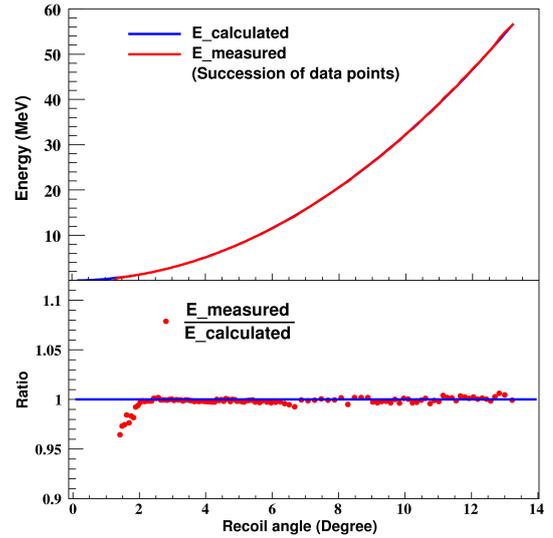
Fig. 53: (upper part) The blue line and red data points show the expected energy curve and measured energy of recoil protons as a function of recoil angle, respectively. The ratio between the measured to expected energy in a given strip is presented in the lower frame.
