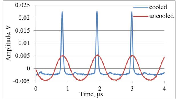
Fig. 23: Proton bunch shortening during electron cooling with 200 mA. Shown are the bunch shapes for the cooled and uncooled proton beam as reported by the bunch phase monitor.
