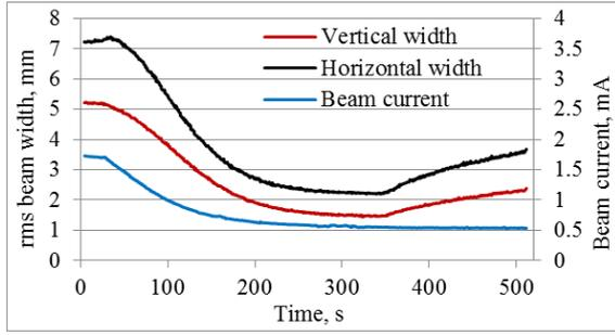
Fig. 21: Evolution of horizontal and vertical beam width and beam current. The 200 mA electron beam was turned on at  $t = 30$  s and turned off at  $t = 350$  s.
