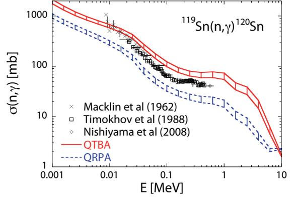
Fig. 62: Radiative neutron capture cross section for  $^{120}\text{Sn}$ .
