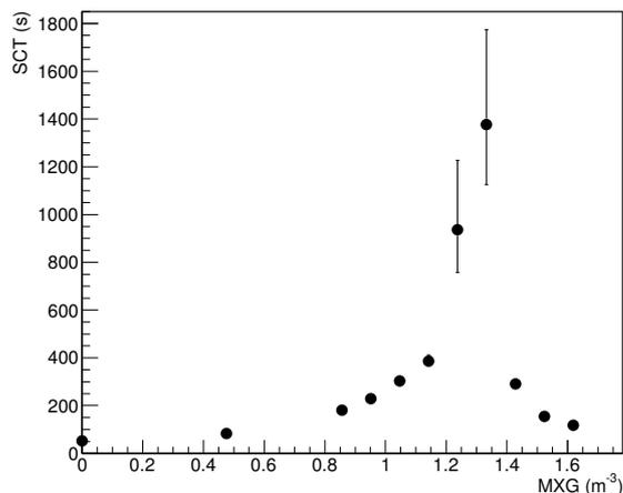
Fig. 32: Measurements of the exponential horizontal polarization lifetime for a series of MXG sextupole settings. The values go through a maximum for sextupole values near  $1.3 / \text{m}^{-3}$ . The best values exceed 1000 s.
