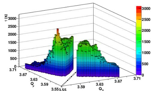
Fig. 17: Beam lifetime as a function of the working point  $(Q_x, Q_y)$ . The beam lifetime increases with decreasing tune difference  $\Delta Q = Q_x - Q_y$ . The exact condition  $\Delta Q = 0$  (dashed line) could not be reached because of coupling.
