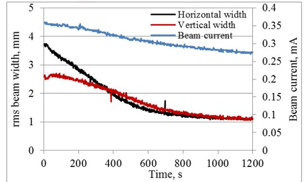
Fig. 24: Evolution of the beam width and proton beam current during electron cooling with 320 mA.
