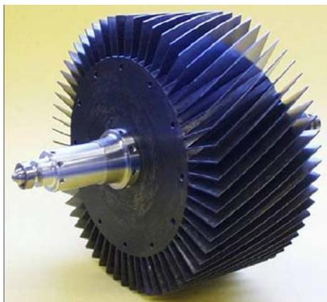
**Fig. 5.6:** Drum of a velocity selector made from a light-weight, neutron absorbing alloy (MgLi). A velocity selector works on the "screw thread principle": it is rotating at high speeds and only neutrons in a certain velocity band can travel undisturbed in the channels between the absorbing partition walls; neutrons outside this velocity band are stopped in the walls. Thus only a certain velocity- or wavelength band can pass this device.
