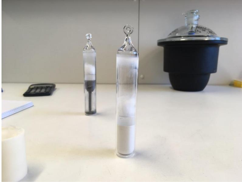
**Figure 16:** Synthesis variant A. The tubes contain the sample before the melting process.
