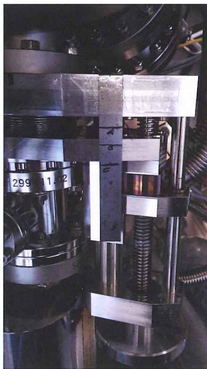
Figure 4.5 – The left side of the picture shows a part of the deflection section of the sputter gun. The label is mounted on a linear transfer flange, which can adjust the distance between sputter gun and sample.
