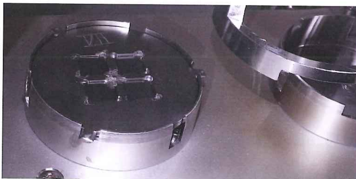
Figure 4.11 – The sample should be put on the trolley in this orientation for every sputtering. The 'ear' of the sample holder, which is perpendicular to the sample edge, is put on the right side.
