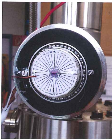
Figure 4.10 – The paper with marks is stuck on the center of the rotator, which does not rotate during rotation. A small rod is fixed at the outer shell, which can be rotated with the rotator. With the indicated degrees, the rotation angle can be known.
