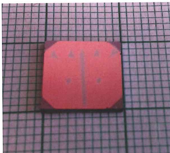
Figure 4.13 – The line was sputtered to know whether the sample is right orientated. The dots are used to check the center of the sample.
