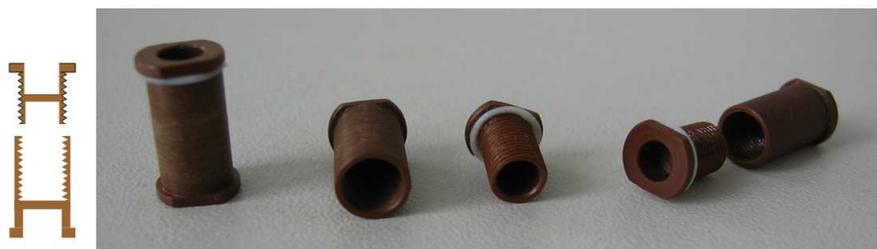
Figure 5.1.3.: Sample holder designed for measurements of liquid samples using the MPMS. The drawing on the left represents a cut through the sample holder. A technical drawing including all measures can be found in the Appendix C.2.
