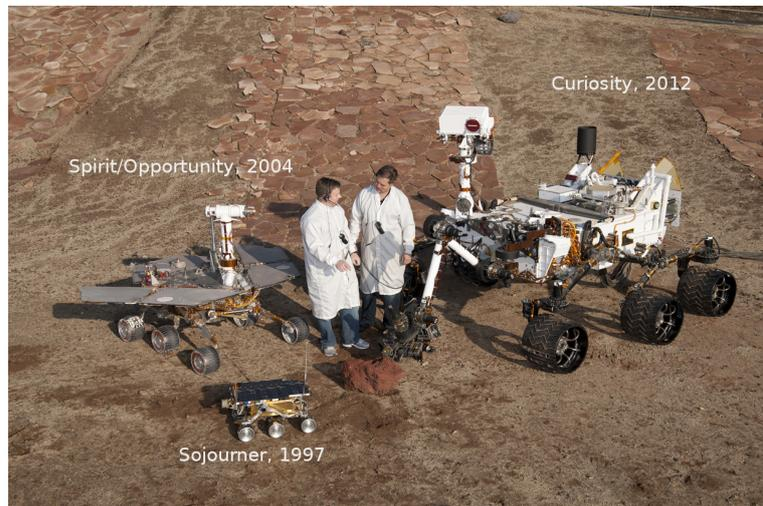
**Figure 1.2:** Two test rovers and a flight spare provides a graphic comparison of three generations of Mars rovers developed at NASA's Jet Propulsion Laboratory, Pasadena, California. (Image credit: NASA/JPL-Caltech)
