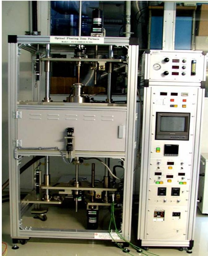
Figure 6.3: FZ furnace operated at FZJ GmbH, Germany.
