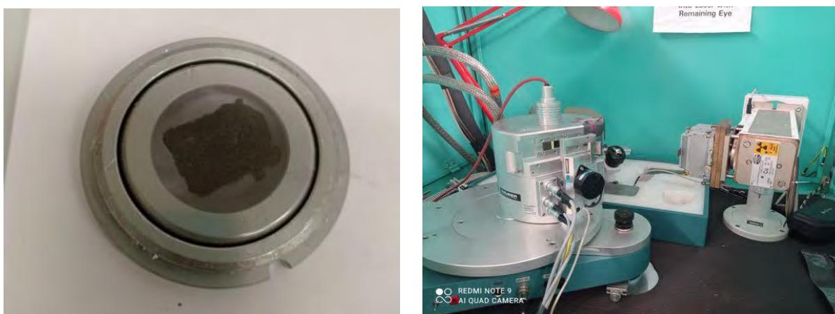
**Fig.5.5 (left) Powder sample inserted in sample holder to be used in x-ray diffraction experiment, (right) The Huber G670 diffractometer system in JCNS-2.**
