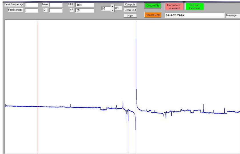
Image 37: RUS spectrum of "fail" steel shown in RUS reduction program
