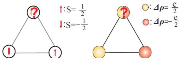
**Figure 1.1 Spin and charge frustration on a triangular lattice. On a triangle with antiferromagnetic interactions, two of the spins are aligned antiparallel, the third one cannot align opposite to both other spins and creates geometric magnetic frustration. The same principle works for charge ordering. Taken from [de Groot, 2012].**
