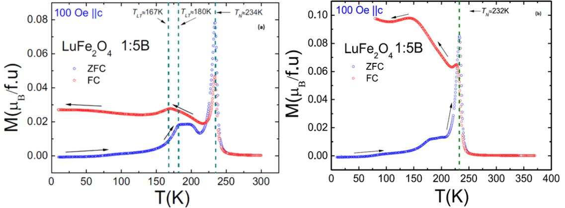
**Figure 3.6: Magnetization  $M(T)$  of  $\text{LuFe}_2\text{O}_4$  single crystals, measured under 100 Oe magnetic field for 1:5 crystal before (left), and after heating up to 400 K (right). [Williamson, 2012].**
