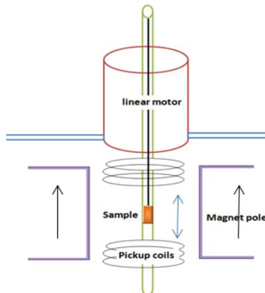
**Figure 2.9 VSM option of the PPMS setup.**
