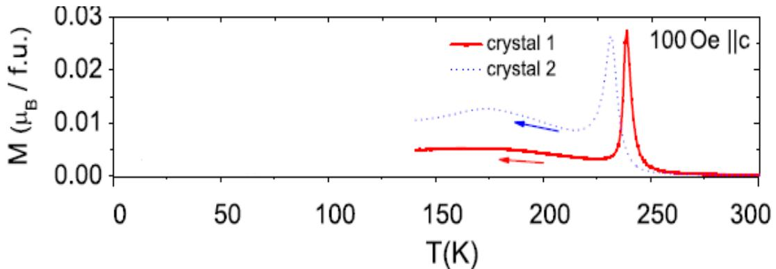
**Figure 3.8** The magnetization ( $M$ ) plotted vs. temperature ( $T$ ) of  $\text{LuFe}_2\text{O}_4$  single crystals measured with an applied magnetic field of 100 Oe. Reproduced from [de Groot et al. 2, 2012].
