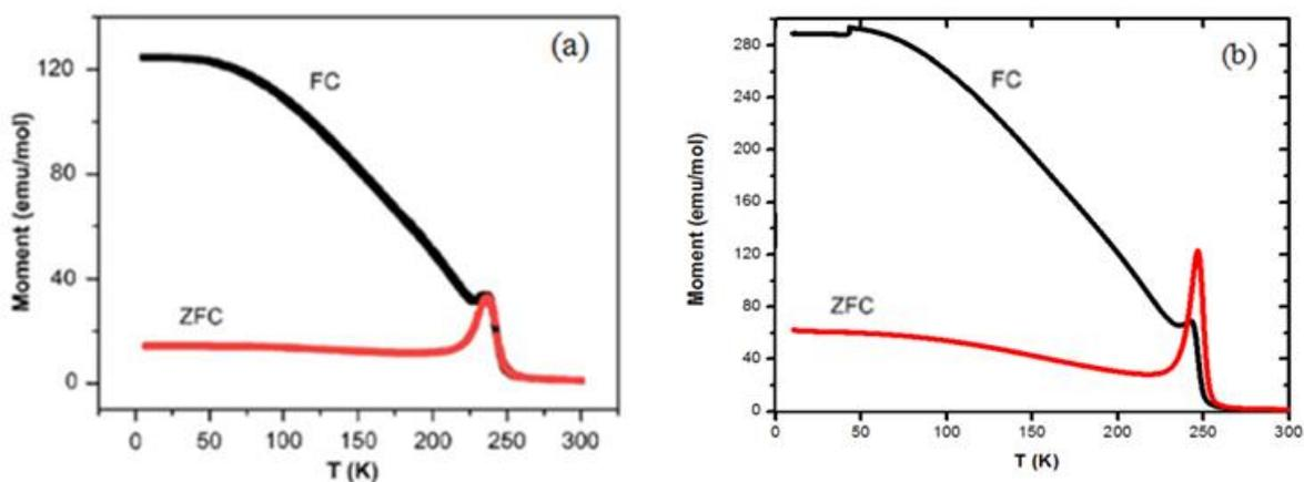
**Figure 3.10** ZFC and FC magnetization measured for polycrystalline  $\text{Lu}_{0.5}\text{Y}_{0.5}\text{Fe}_2\text{O}_4$  in an external field of 100 Oe (a) Serrao's sample. Taken from [Serrao et al., 2008]. (b) S6 sample.
