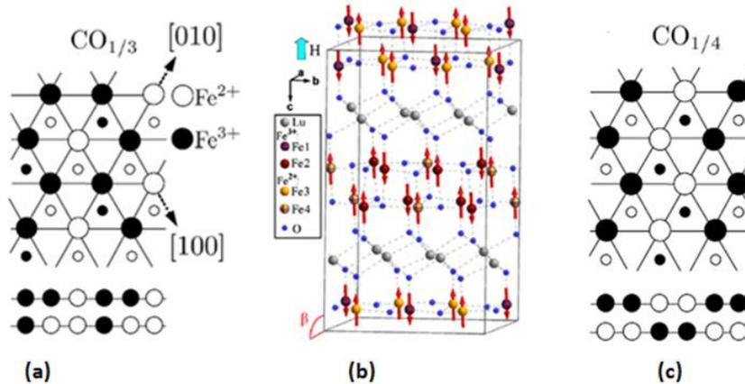
Figure 1.7 (a) Proposed ferroelectric charge configuration in Fe/O bilayer in  $\text{RFe}_2\text{O}_4$  (Fe ions in upper/lower layer are drawn as large/small circles). Taken from [Naka et al., 2008]. (b) The experimentally established CO pattern of  $\text{LuFe}_2\text{O}_4$ . Taken from [de Groot et al. 1, 2012]. (c) An alternative CO that has been considered theoretically. Taken from [Naka et al., 2008].
