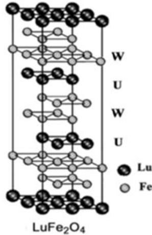
Figure 1.6 LuFe<sub>2</sub>O<sub>4</sub> crystal structure. Taken from [Qin et al. 1, 2009].
