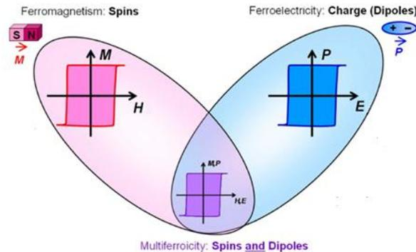
**Figure 1.2 ME Multiferroics combine both ferroelectricity and magnetism represented by the overlapping area, the coupling between these orders leads to a ferroelectric response to a magnetic field and vice versa. Taken from [de Groot, 2012].**
