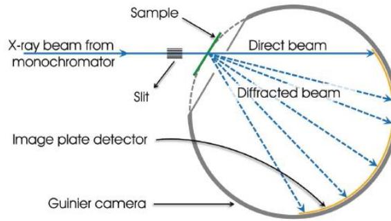
**Figure 2.7 Transmission geometry powder diffraction. Taken from [Kumar, 2012].**
