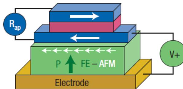
**Figure 1.3 Multiferroics RAM. The information is stored by the magnetization of the two blue layers and is read out by GMR, but with the insertion of a Multiferroics (green) layer, the information is stored by applying a voltage. Taken from [Bibes and Barthélémy, 2008].**
