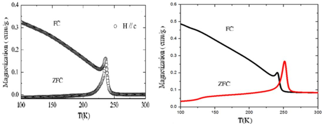
Figure 3.9 ZFC and FC magnetization in external fields of 10 Oe for measured (left panel) single crystal  $\text{LuFe}_2\text{O}_4$  Wang's sample. Reproduced by [Williamson, 2012] from [Wang et al., 2009]. (Right panel) polycrystalline S5  $\text{Lu}_{0.5}\text{Y}_{0.5}\text{Fe}_2\text{O}_4$  measured with 100 Oe.
