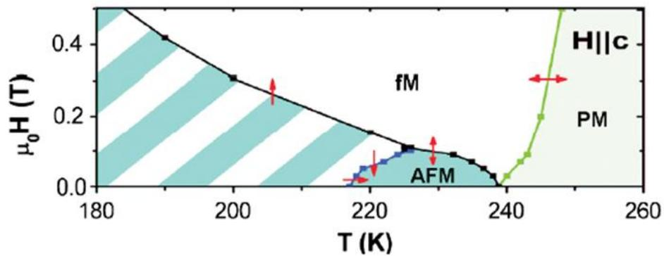
Figure 3.15 H-T phase diagram of  $\text{LuFe}_2\text{O}_4$ . Taken from [de Groot et al. 2, 2012]. In the hatched region, the AFM phase is stable when reached by increasing H after zero-field cooling and the fM phase is stable when reached by decreasing the field from high values.
