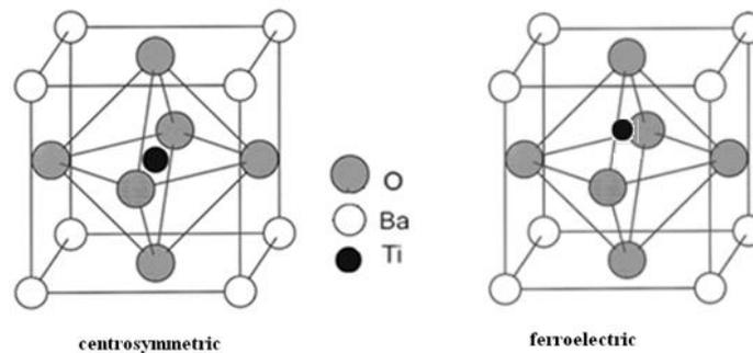
Figure 1.4 Traditional mechanism of ferroelectricity in BaTiO<sub>3</sub>, off center displacement of Ti ion to drive ferroelectricity. Left side figure taken from [Hill, 2000].
