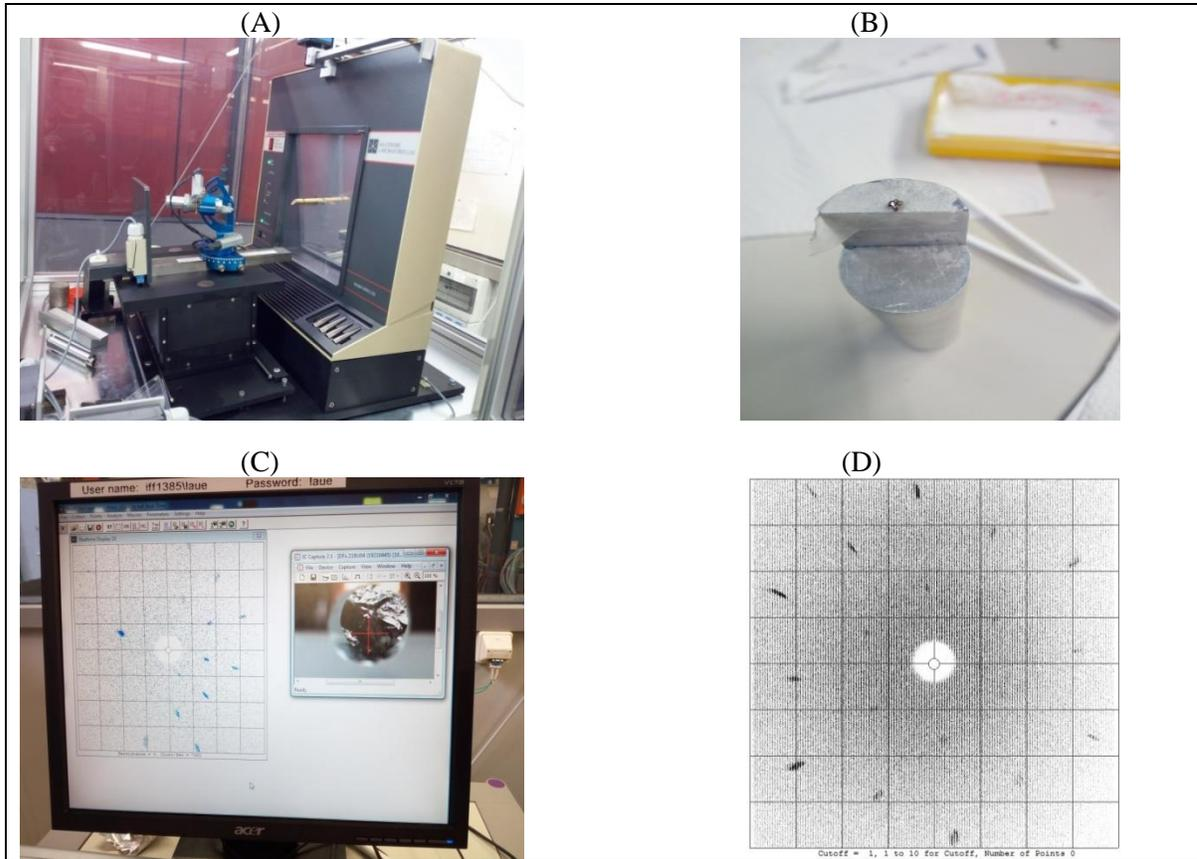
**Figure 3.7:** (A) Photo of the MWL100 Camera System (B) the crystal fixed on the holder (C) a screenshot of the control software (D) an image from the Laue camera for the crystal of  $\text{MnFe}_4\text{Si}_3$  oriented along the c-axis.
