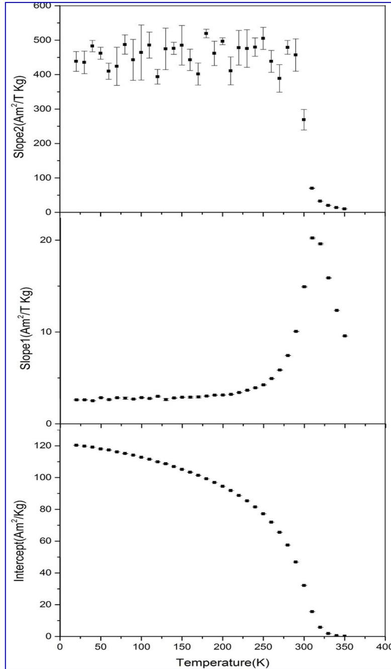
**Figure 4.4:** Bottom: magnetization in the saturation region; Middle: slopes in the saturation region; Top: slopes in the region near zero field,  $H \parallel [100]$ . Error bars are shown if they exceed the symbols size.
