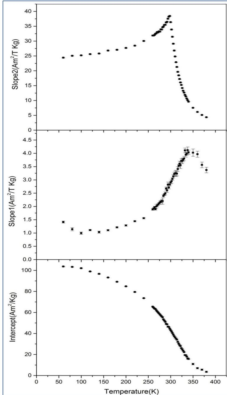
**Figure 4.7: Bottom: magnetization in the saturation region; Middle: slopes in the saturation region; Top: slopes near zero field region.  $H \parallel [001]$ . Error bars are shown if they exceed the symbols size.**
