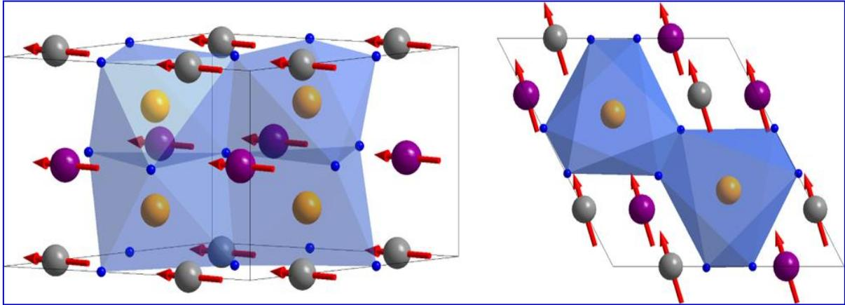
**Figure 2.9:** Schematic diagram illustrating the ferromagnetic structure of  $MnFe_4Si_3$  at 200 K in magnetic space group  $Pm'$ . Left, slightly tilted projection approximately along  $[110]$ -direction; right, projection along  $[001]$ -direction [Hering et al., 2015].
