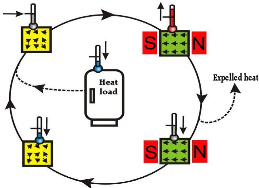
Figure 2.1: Schematic of a magnetic-refrigeration cycle [Brück, 2005].
