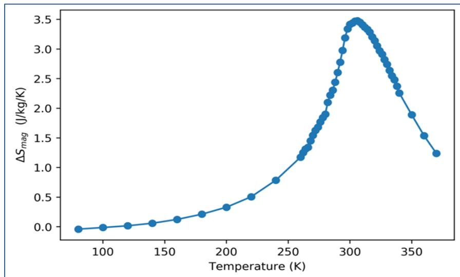
**Figure 4.11:** MCE of  $\text{MnFe}_4\text{Si}_3$  calculated from the temperature-dependent magnetization at a field of 6T ( $\mathbf{H} \parallel [001]$ ).
