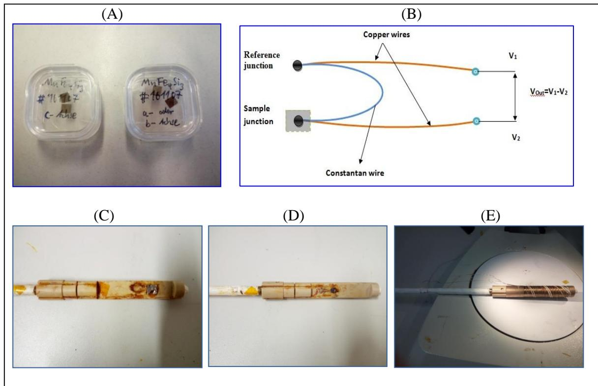
**Figure 3.15: The experimental setup: (A) the four samples used in these measurements (B) a schematic drawing of the thermocouple (C) the holder with the samples mounted (D) the back side of the holder with the reference junction installed (E) the holder with the heater placed around the sample.**
