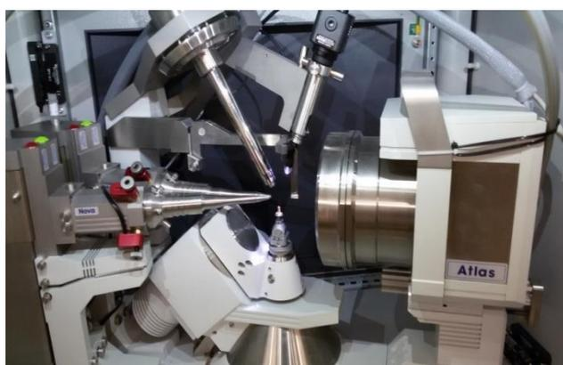
**Figure 4.4: The Agilent Supernova diffractometer at Forschungszentrum Jülich**
