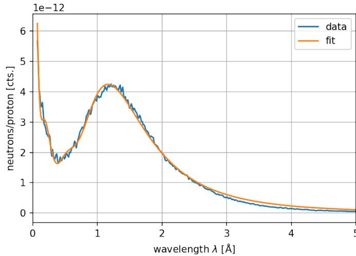
Figure 51: Spectra at a moderator temperature  $T_{mod} = 140 \text{ K}$  fitted with eq. 25.
