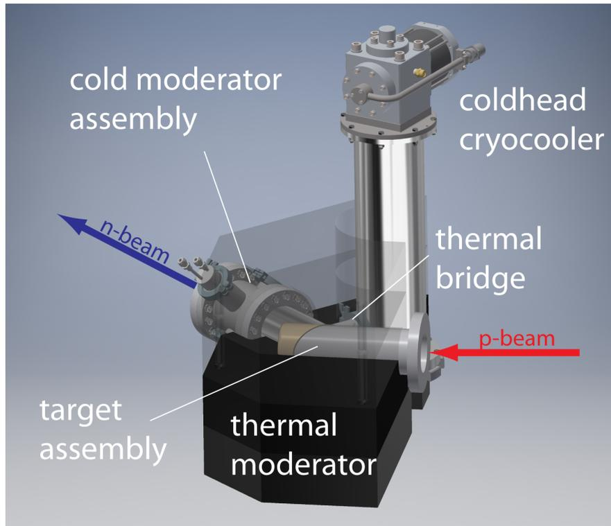
Figure 14: Rendering of the thermal moderator assembly.
