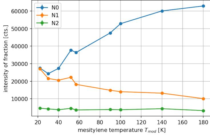
Figure 52: Intensities of the different neutron populations of the three Maxwell-Boltzmann distributions obtained by fitting to measured spectra (fig. 48) of frozen mesitylene ( $T_{mod} \leq 180$  K) and plotted in dependence of  $T_{mod}$ . The fit errors are fully covered by the size of the markers.
