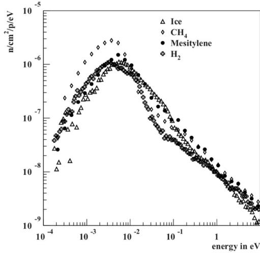
Figure 8: Neutron spectra for ice, solid methane, mesitylene (phase III) and liquid hydrogen measured at 20 K in the JESSICA experiment [19].
