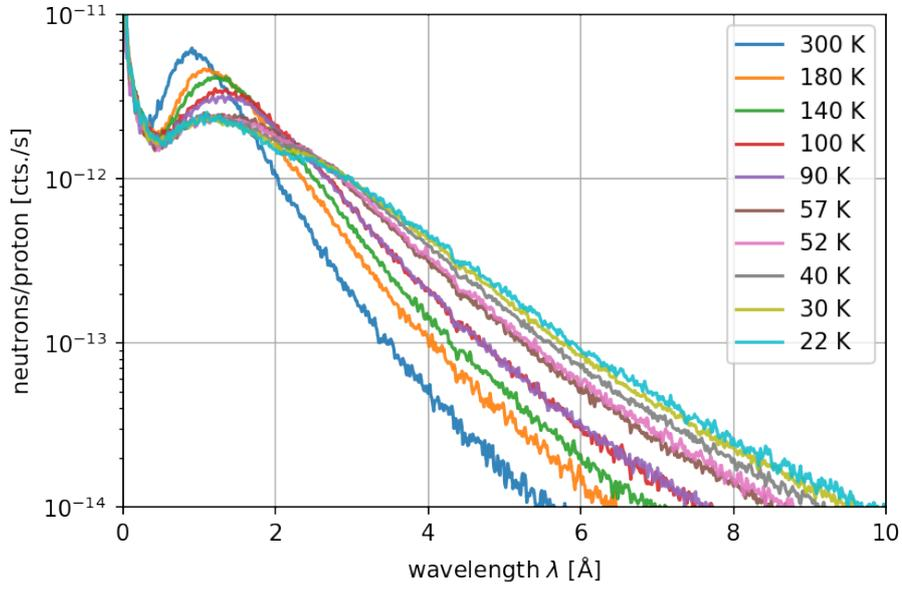
Figure 48: Spectra of the summed up and corrected runs for mesitylene temperatures  $T_{mod}$  in a range from 300 K to 22 K.
