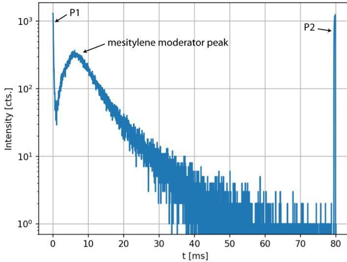
Figure 33: Raw TOF spectra of detector 3 measured at  $T_{mod} = 24\text{ K}$  with a run time of  $t_{run} = 600\text{ s}$ , a frame length of  $t_{fra} = 80.5\text{ ms}$  and a bin width of  $t_{bin} = 25\text{ }\mu\text{s}$ .
