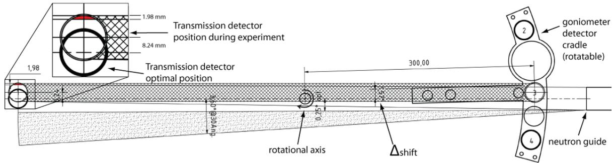
Figure 28: Drawing to scale of the detector assembly. The true position of the transmission detector 1 during the experiment has been determined by turning the goniometer for  $\Delta_{shift} = 1.57^\circ$  from  $0^\circ$  position.
