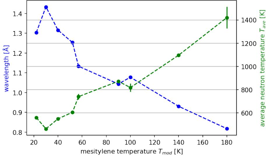
Figure 54: Weighted average neutron temperature and corresponding wavelengths of the three Maxwell-Boltzmann distributions plotted in dependence of  $T_{mod}$ .
