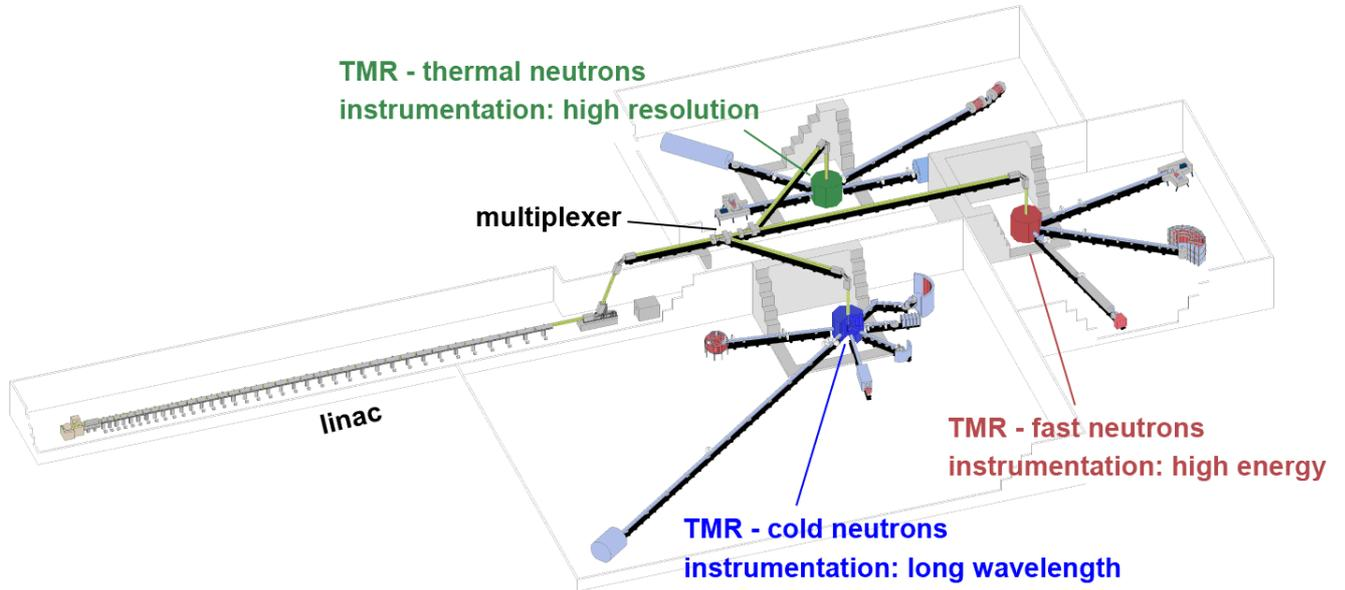
Figure 1: HBS baseline design with the central components. The linac (linear accelerator) for the production of a proton beam, the multiplexer to distribute the proton beam, the TMR (target-moderator-reflector) stations surrounded by a safety shielding and an exemplary instrumentation [11].
