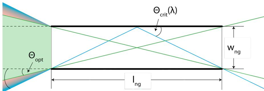
Figure 39: The top view sketch of the neutron guide shows exemplary (i) the divergence angle  $\Theta_{opt}$  for the optical acceptance (green) and (ii) the wavelength dependent acceptance (color gradient from red for higher wavelengths to blue for lower wavelengths) given by the critical angle  $\Theta_{crit}(\lambda)$ .
