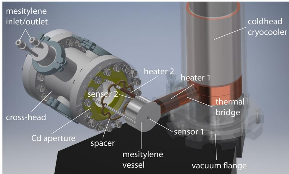
Figure 15: Rendering of the cold moderator assembly.
