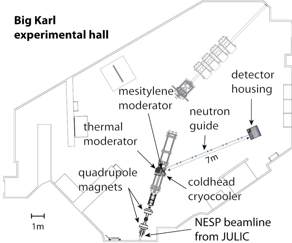
Figure 10: Big Karl experimental hall with assembled mesitylene moderator experiment setup (true to scale).
