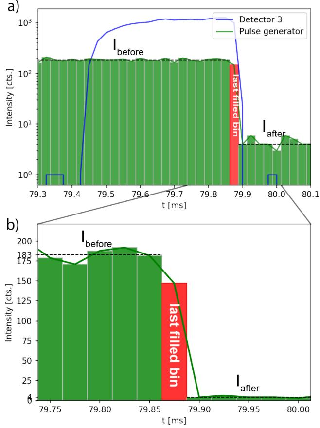
Figure 34: Bar plot of the pulse generator signal magnified for P2. The red marked bin shows the last, partially filled bin for TOF repetitions with  $T_{mic}$ . The dashed lines displays the average intensities before and after P2. In the semi logarithmic plot a) the blue line shows P2 measured by detector 3. b) shows the magnified area around the last filled bin.
