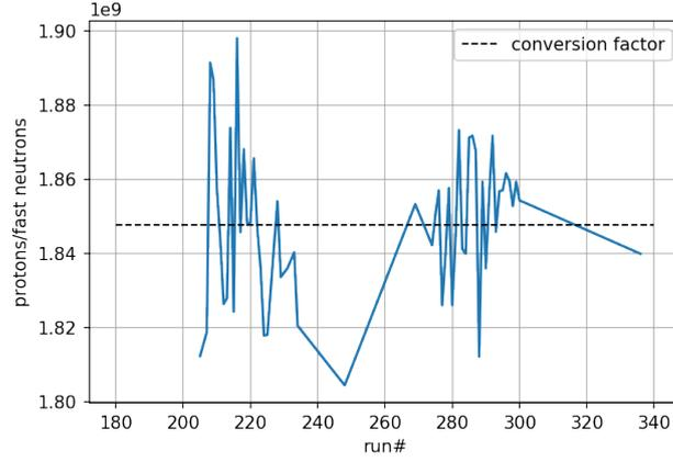
Figure 46: Plot of the quotient  $I_p/I_{fn}$  against the run# of the experiment "IH<sub>2</sub>". The dashed line shows the conversion factor  $C_{conv}$ .
