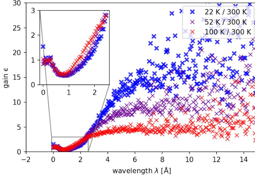
Figure 49: Intensity gain factor  $\epsilon$  for 22 K, 52 K and 100 K normalised to the room temperature spectrum (300 K) plotted in dependence of  $\lambda$ . The inset shows the low  $\lambda$  region.
