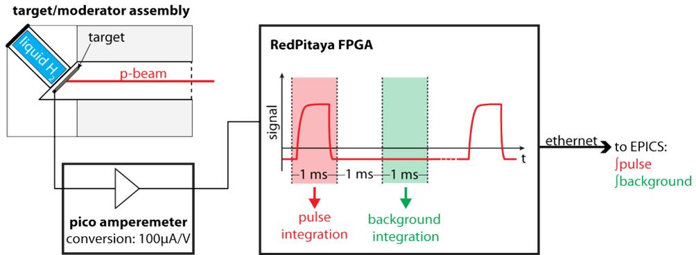
Figure 43: Sketch of the current measurement setup used since the second half of the experiment "lH<sub>2</sub> moderator". The Ta target is connected to a picoamperemeter to amplify and convert the current to a proportional voltage signal. The signals of proton pulse and background are separately integrated by a RedPitaya FPGA and stored in EPICS.
