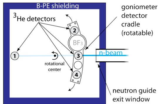
Figure 26: Illustration (not true to scale) of the detector assembly mounted inside the B-PE shielding. The light blue beam illustrates the shading of the <sup>3</sup>He transmission detector 1 by detector 3 in the front position.
