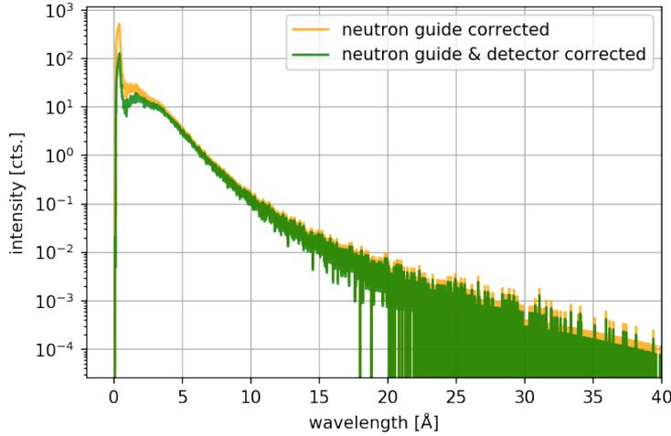
Figure 42: Rescaled, re-binned and neutron guide corrected spectra (see also fig. 41) plotted in blue before  $^3\text{He}$  detector correction and after in green.
