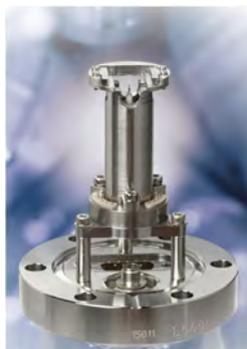
*Integrating the KoalaDrive™ nanopositioner as coarse approach inside a tube scanner pushes the design of SPMs towards ultra compact instruments. A minimal size leads to improvements of the key figures of merit in scanning probe microscopy. A smaller size leads directly to a smaller thermal drift and increases the eigenfrequencies, leading to a better damping of external vibrations.*
