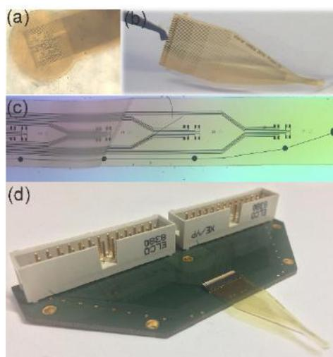
FIG. 6: Optical images of freely standing graphene-based probes (a-c) and as bonded to a special carrier for in vivo use (d).
