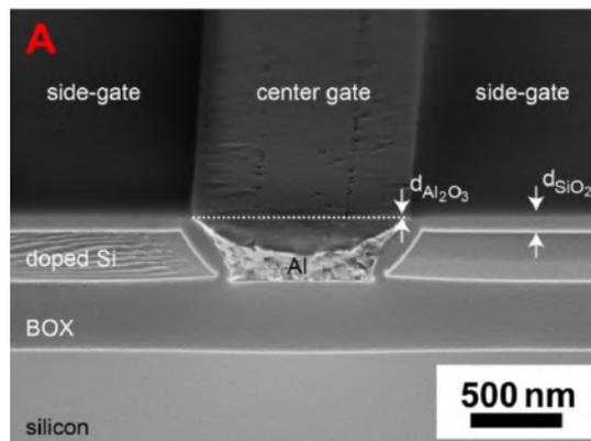
FIG. 1: SEM image of the buried tri-gate structure.
