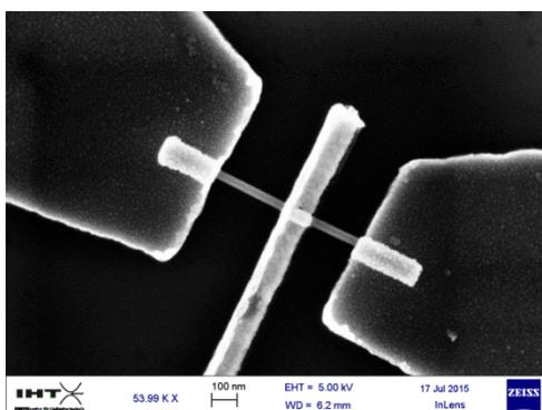
FIG. 5: InAs/GaSb Core-shell NW. AZ 726 MIF used to etch away the GaSb-shell below the center contact.
