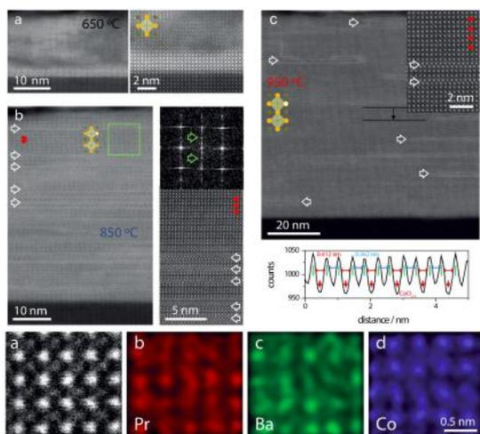
FIG. 4: HR(S)TEM analysis of atomic structure and ordering in PBCO thin films, revealing atomic ordering in the  $\text{CoO}_{2-\delta}$  atomic planes (top right), while scanning EDX analysis (bottom panel) shows no sign of ordering in the A-site cation sublattice.
