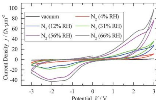
FIG. 4: Cyclic voltammograms of Pt/HfO<sub>2</sub>/Pt from vacuum to 66 % RH Adapted from [4].
