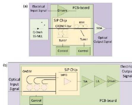
FIG. 1: DWDM transceiver block diagram. (a) Tx side. (b) Rx side.
