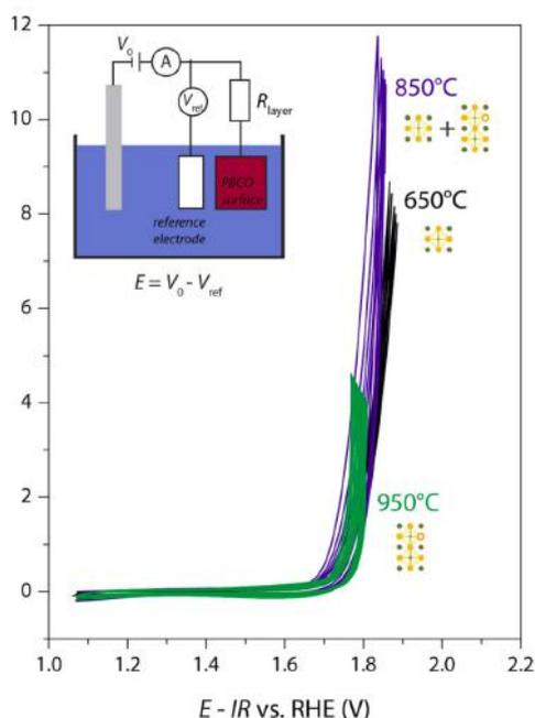
FIG. 5: Electrocatalytic performance of different polymorphs of PBCO, showing activity for OER, but no sign of improved performance in oxygen-vacancy-ordered catalyst layers. This way atomic structure and band alignment can be discarded as main descriptor of catalysis of OER during water splitting operation.
