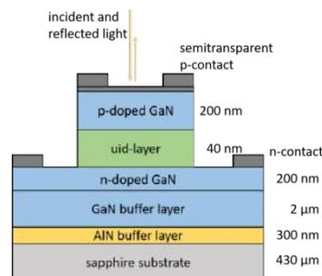
FIG 1: Structure of the device
