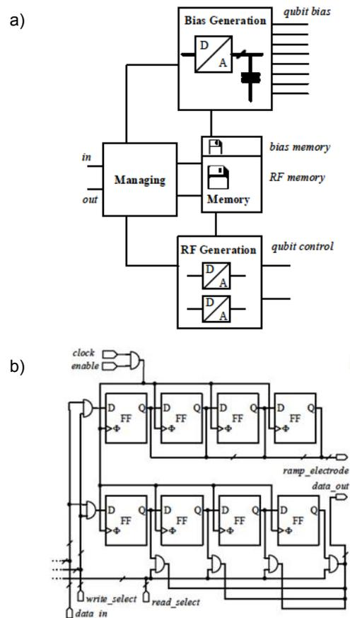
FIG. 1: a) Block diagram of the control electronics for one qubit. b) Structure of two registers of bias memory with four-bit resolution.
