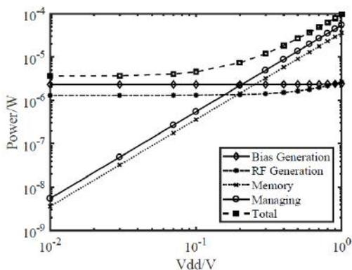
FIG. 2: Power consumption of the control electronics during qubit operation as function of the voltage supplied to the digital circuit elements  $V_{dd}$
