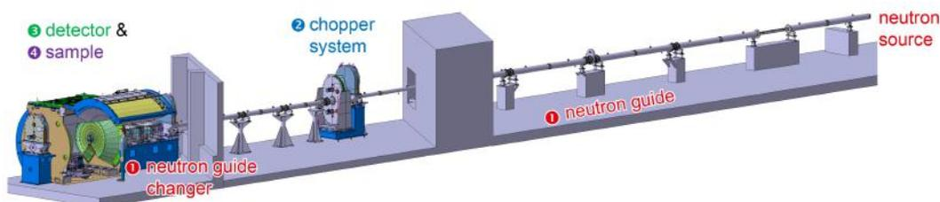
FIG. 1: The POWTEX instrument and its main instrument components.
