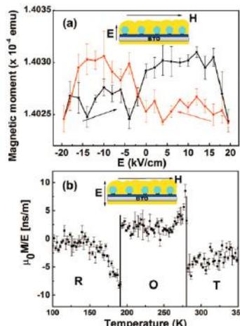
FIG. 3: (a) Magnetic moment vs. applied electric field of the sample Au/BTO/Ti/NP/Au at 300 K and 5 mT. The black data points were measured with increasing DC field from -20 to +20 kV cm<sup>-1</sup>, the red data points were measured in the reversed sequence (b) ME coefficient  $\alpha$ ME vs. temp. measured in an AC electric field with
