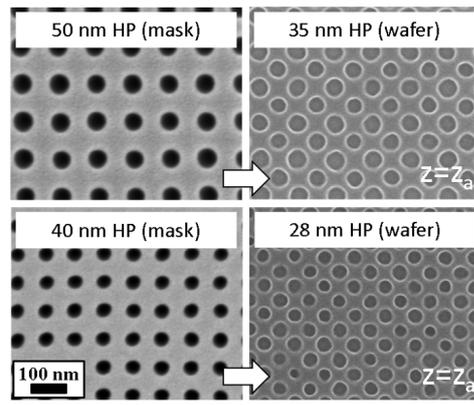
FIG. 4: Typical exposure results in achromatic Talbot distance. Compared to the mask half-pitch, the wafer half-pitch is reduced by a factor of  $\sqrt{2}$  (and tilted by  $45^\circ$ ).
