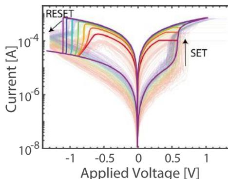
FIG. 3: Comparison of the simulated  $I$ - $V$  curves to the experimentally measured  $I$ - $V$  curves of the device. The simulation shows all trends and verifies the assumption of an internal series resistor caused by the  $\text{TiO}_x$  layer.
