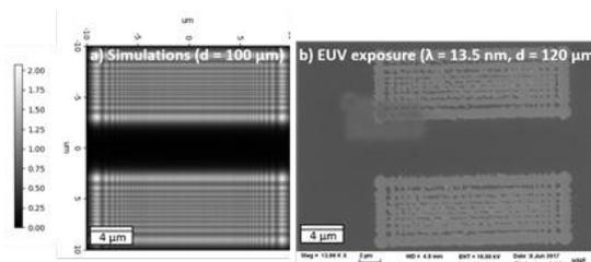
FIG. 4: Comparison between simulated intensity distribution at wafer plane (a) and exposure result (b) of two rectangles (8  $\mu\text{m} \times 20 \mu\text{m}$ ).
