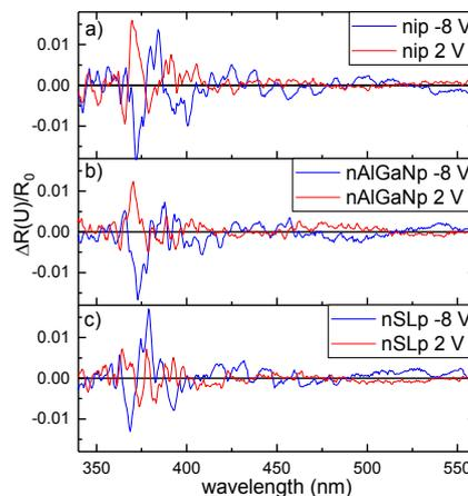
FIG 3: Change of reflectivity by applied bias voltage for: a) n-i-p, b) nAlGaNp and c) nSLp.
