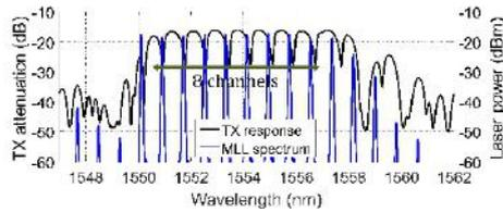
FIG. 2: Tx transmission and filtered MLL spectra at 25 °C and 257 mA showing 8 RRM channels aligned within the pass-band of the CROW filter.
