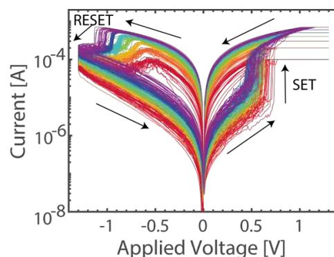
FIG. 1: *I-V* switching curves for a set of current compliance values. Voltage sweeps between -1.3 V and 1.3 V were performed with current limitation at positive polarity varied from 100 μA (red curve) to 700 μA (violet curve).
