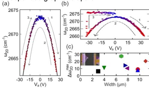
FIG. 2 (a)  $\omega_{2D}$  versus  $V_a$  shows parabolic behavior. The gray arrows 1 to 3 indicate the sweep direction of the potential  $V_a$  in the measurement. (b) Similar to Fig. 2a, but for a device of which the graphene ruptured while approaching  $V_a = -24$  V. (c) The maximum relative shift of  $\omega_{2D}$  before mechanical failure for the devices measured in this work.
