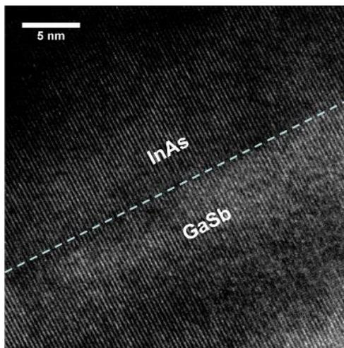
FIG. 4: HRTEM image of the InAs/GaSb interface.
