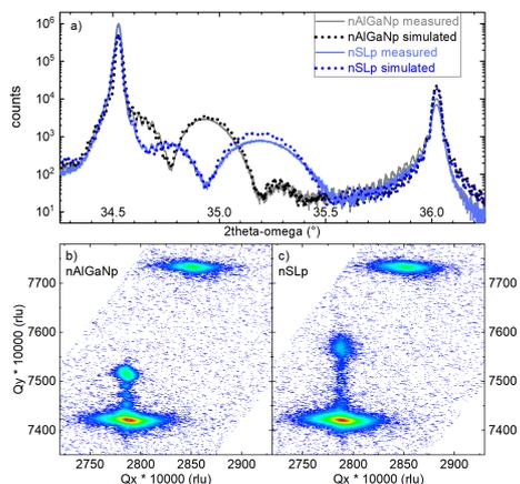
FIG 2: a) Measured (solid lines) and simulated (dashed lines) (002) reflex of nAlGaNp and nSLp, (105) reciprocal space map of b) nAlGaNp and c) nSLp
