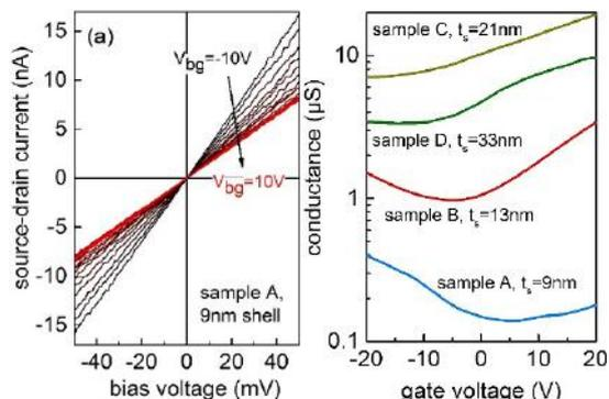
FIG. 3: (a) Gate-dependent IV curves of a GaAs/InSb nanowire with a core radius of 40nm and a shell thickness of 9nm. (b) Transconductance curves of four wires with different shell thicknesses.
