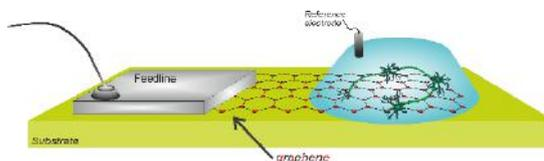
FIG. 3: Schematics of a liquid-operated GMEA.
