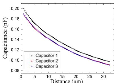
FIG. 2: Capacitance curves of the three sensors during mask approach to the substrate (points) with fit curves  $C(d) = a + \frac{b}{c+d}$  (lines)
