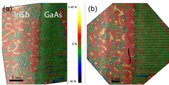
FIG. 2(a,b): HRTEM images for different nucleation spots of InSb on GaAs, superimposed by GPA strain maps. All of them show an abrupt compensation of the lattice mismatch induced strain close to the interface.
