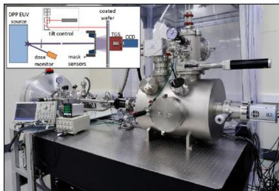
FIG. 1: Photograph of the EUV Laboratory Exposure Tool (EUV-LET). The main components are labeled in the schematic drawing (inset).
