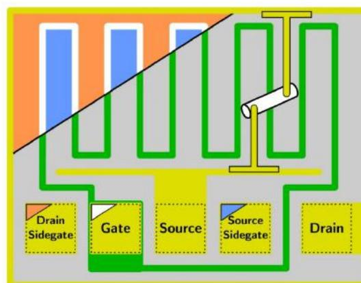
FIG. 2: Meander layout with contact pads and NW illustrated.
