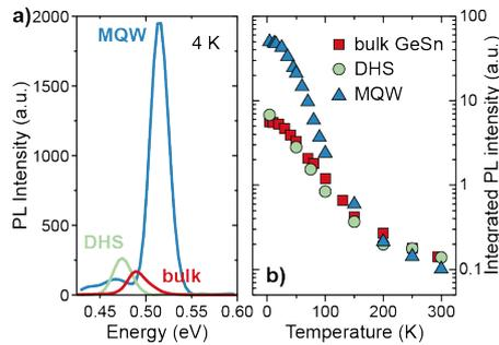
FIG. 2: a) Comparison of photoluminescence spectra at 4 K. b) Temperature-dependent PL for different structures.
