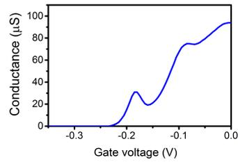
FIG. 3: An example of transimpedance characteristics of one split gate of the gated double quantum dot in a wafer with InAs layer. Oscillations in the transimpedance reveal disordered electrostatic potential landscape.
