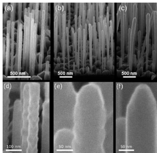
FIG. 1: Overview and zoomed-in SEM micrographs of GaAs/InSb core/shell nanowires with a shell growth time of 5 min (a,d), 30 min (b,e) and 90 min (c,f).
