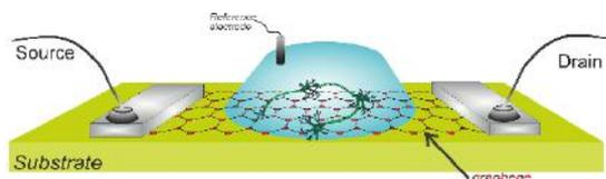
FIG. 1: Schematics of a liquid-gated GFET.
