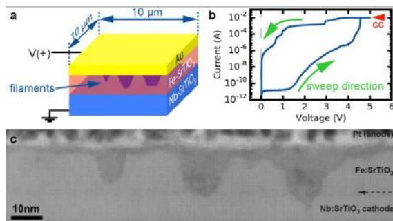
FIG. 1: (a) Scheme of the device, (b) Electroforming I-V curve, and (c) Annular bright-field STEM image simultaneously showing multiple conducting filaments with darker contrast than the matrix.
