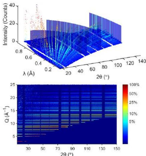
FIG. 2: Top: Three-dimensional plot of an angular- and wavelength-dispersive data set of diamond obtained from the POWGEN instrument (SNS, Oak Ridge). Bottom: Two-dimensional color-coded  $Q$  vs.  $2\theta$  plot of the same data set.
