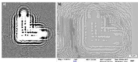
FIG. 3 Comparison between simulated (a) and fabricated (b) elbow test structure.
