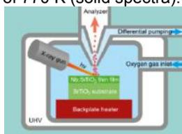
FIG. 1: Schematic illustration of the sample stack as well as the near ambient pressure X-ray photoelectron spectroscopy measurement setup.[3]
