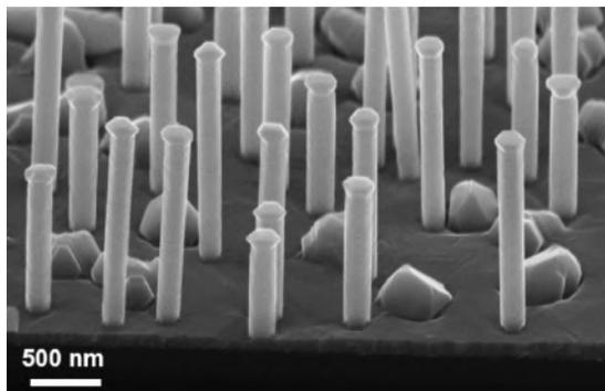
FIG. 3: SEM micrograph InAs/GaSb core-shell NWs.
