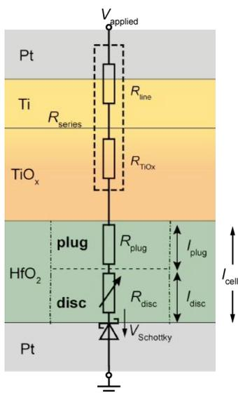
FIG. 2: Equivalent circuit diagram for the electrical model of the Pt/ $\text{HfO}_2$ / $\text{TiO}_x$ /Ti/Pt device. The voltage is applied to the top electrode.  $V_{\text{Schottky}}$  equals the reverse voltage across the diode.
