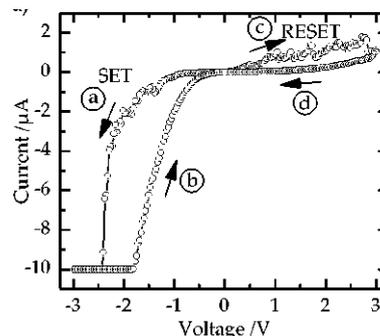
FIG. 4:  $I$ - $V$  curve recorded on a  $\text{TiO}_2$  NP monolayer exhibiting bipolar resistive switching (BRS) properties. The arrows and letters besides the plotted curves depict voltage sweep direction. Reprinted from [3].
