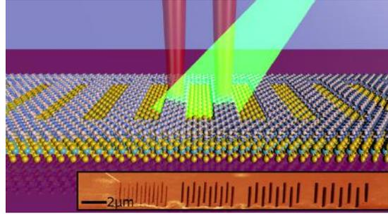
FIG. 4: Schematic of a TMDC-ML covered with h-BN nanoribbons. Inset: AFM measurement of a nano-patterned h-BN cover flake.
