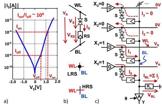
FIG 1: Elements of a memory architecture. a) exemplary I/V characteristics of a selector device [6]. b) Memory cell, composed of a selector S connected to a word line WL and an RS connected to a bit line BL. A HRS isolates WL and BL while a LRS establishes an unidirectional connection between WL and BL. c) bit line architecture and current summation.
