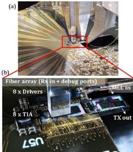
FIG. 3: (a) Photograph of transceiver board with optical I/O. (b) Detailed view of the silicon photonics chip and high speed components.
