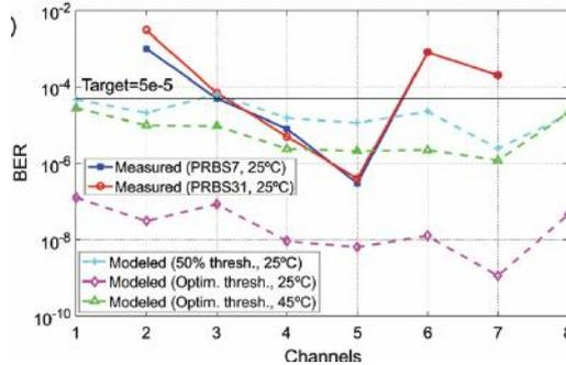
FIG. 4: Measured BER using the full transceiver at 14 Gbps for PRBS  $2^7-1/2^{31}-1$  and modeled BER
