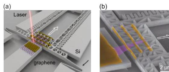
FIG. 1 (a) Schematic illustration of a comb-drive actuator that applies uniaxial strain to the graphene flake by moving in the direction of the white arrow. The fixed part is resting on the substrate whereas the suspended part is freely hanging and is held by V-shaped springs (see black arrow). (b) False color scanning electron microscope (SEM) image of a measured device, in which the cross-linked PMMA clamping (yellow) of the graphene (pink) is highlighted.
