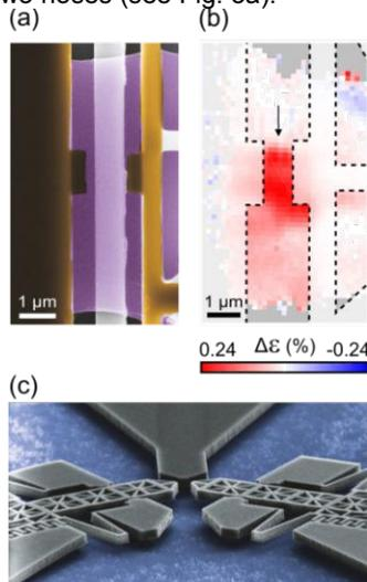
FIG. 3 (a) False color SEM image (similar to Figure 1b) of a typical measured device where the PMMA-clamping contains two noses. (b) The spatially resolved induced strain  $\Delta\epsilon$  shows a maximum gradient ( $1.4\%/um$ ) at the position of the black arrow. (c) False color SEM image of a device used for triaxial strain fields.
