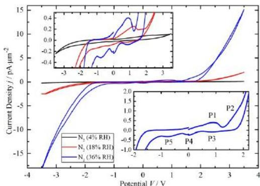
FIG. 2: Cyclic voltammograms (CV) of Pt/Ta<sub>2</sub>O<sub>5</sub>/Pt in nitrogen atmosphere for relative humidity values from 4 % to 36 %. Each CV shows the third sweep. Upper left inset: Zoom showing detailed redox peaks at the different conditions. Lower right inset: Numbering of the observed peaks after initial cycling in tantalum oxide system [4].
