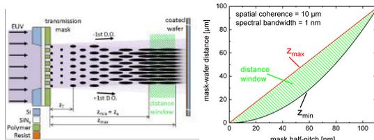
FIG. 3: Schematic drawing of achromatic Talbot lithography approach (left). Calculated distance window for the EUV-LET (right).
