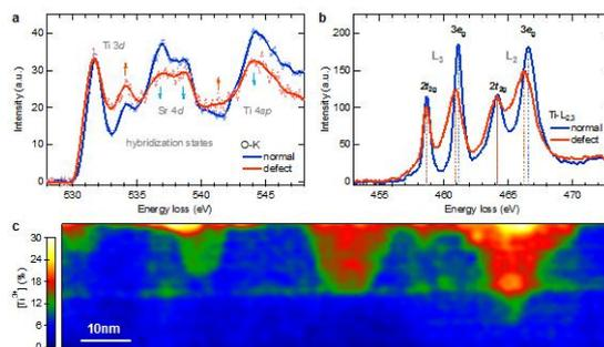
FIG. 2: Electron core-loss spectra of (a) O-K edge and (b) Ti-L<sub>2,3</sub> edge from normal SrTiO<sub>3</sub> and conducting filaments comprising  $Ti^{3+}$ . (c) Distribution map of  $Ti^{3+}$  (atomic percentage).
