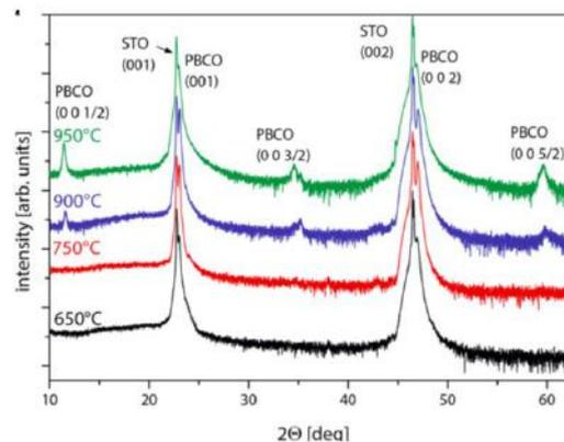
FIG. 3: X-ray diffraction obtained for epitaxial PBCO synthesized at different growth temperature. Half-order superstructure peak occur for samples grown above 900°C indicating atomic ordering.
