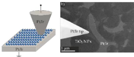
FIG. 3: Schematic illustrations of the (Pt/Ir)/ $\text{TiO}_2$  NP film/(Pt/Ir tip) device (a). Exemplary SEM image of a  $\text{TiO}_2$  NP film on the Pt/Ir surface, exhibiting mono- and multilayers. On the left hand side, the Pt/Ir coated tip electrode is visible (b). Reprinted from [3].
