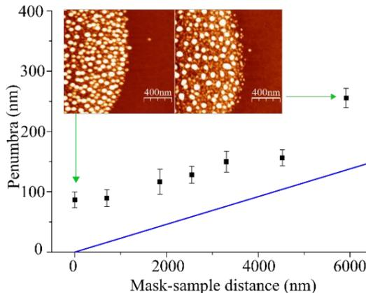
FIG. 3:  $2\sigma$  widths of the error function fitted to angularly averaged profile lines (penumbra) of the deposited Au circles on Si(111) (black data points). The solid blue line gives the penumbra size expected geometrically for a ballistic path of the atoms during MBE growth. Insets: SFM images of the rims of two deposited circles corresponding to the data points at the green arrow.
