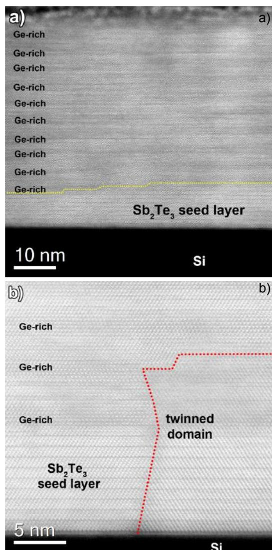
FIG. 1: Z-contrast HAADF STEM images showing a) an overview of the GeTe-Sb<sub>2</sub>Te<sub>3</sub> superlattice with Sb<sub>2</sub>Te<sub>3</sub> seed layer on Si substrate and b) the twin boundary in the Sb<sub>2</sub>Te<sub>3</sub> seed layer.
