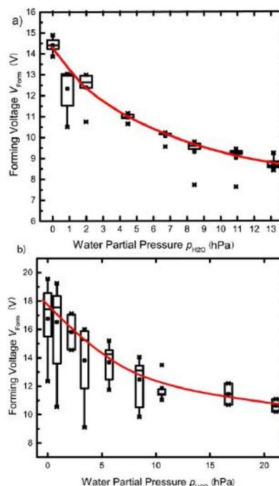
FIG. 1: Forming statistics of a) Ta<sub>2</sub>O<sub>5</sub>(20 nm)/Ta(15 nm) and b) HfO<sub>2</sub>(30 nm)/Hf(20 nm) as function of the water partial pressure in the probing chamber. Adapted from [4].
