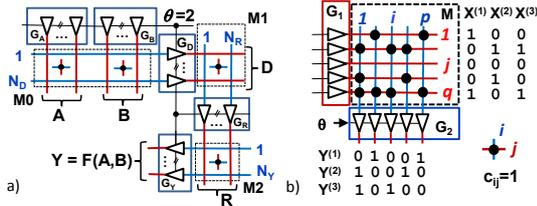
FIG. 2: a) 3-layered BiNAM-architecture for a connection-centric implementation of  $Y=F(A,B)$ , b) example mapping with 3 pairs ( $X^{(k)}, Y^{(k)}$ )
