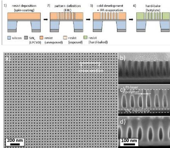
FIG. 2: Top: Process flow for the developed mask fabrication process. Bottom: Top-down SEM image of 30 nm HP mask. Right side: Cross-sectional SEM images of fabricated mask structures with HPs of 30 nm (b), 40 nm (c) and 50 nm (d).
