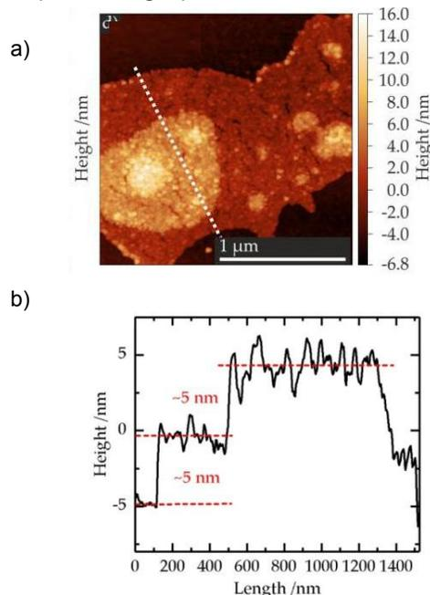
FIG. 2: Exemplary AFM image of a  $\text{TiO}_2$  NP film after transferring to Pt/Ir surface (a) and the corresponding height profile (b). Reprinted from [3].
