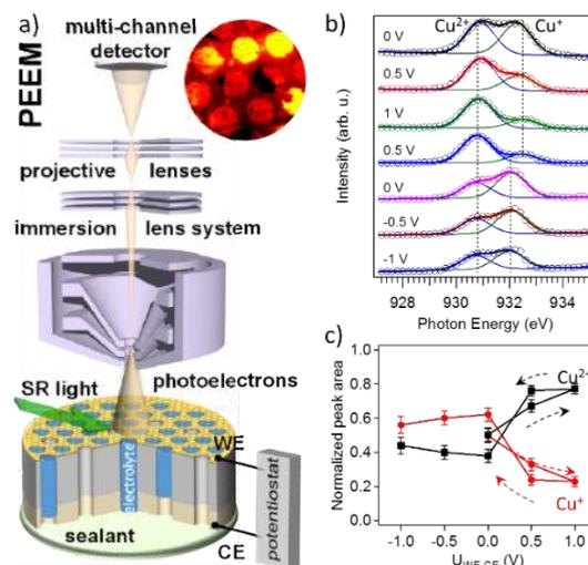
**FIG. 1:** (a) A schematic of the PEEM electrochemical setup; Inset: PEEM image of the graphene capped MCA at the O K-edge energy. Electrolyte filled channels appear brighter compared to dry ones. (b) Averaged XAS Cu  $L_3$ -edge spectra collected from a graphene-capped channel filled with 0.1 mol/l  $\text{CuSO}_4$  solution. (c) Normalized area of the fitted Cu peaks from (b), plotted against the WE potential.
