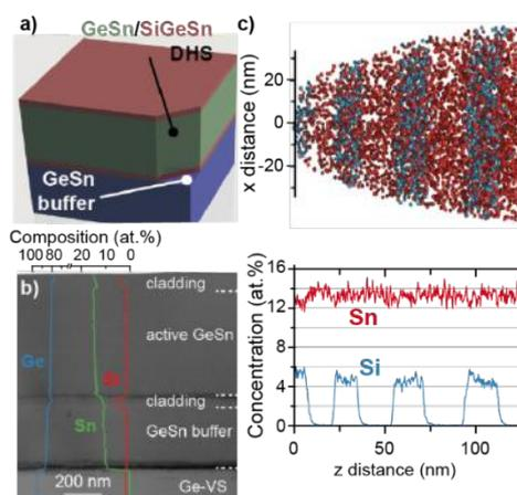
FIG. 1: a) Schematics of the heterostructure material stack. b) Cross-sectional TEM micrograph and overlaid EDX profile of the grown DHS. c) Atom probe tomography (APT) data and corresponding elemental distributions.
