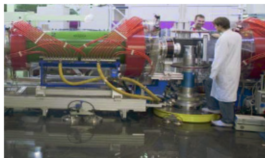
FIG. 1: The sample position (on the right) and second precession coil (green) of the J-NSE spectrometer.
