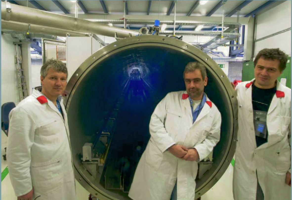
Neutrons show where atoms are and what atoms do: The Jülich Centre for Neutron Science (JCNS) at the IFF was founded in 2006 to operate state-of-the-art neutron scattering instruments at the most modern of highest flux sources in the world. Here: The Small Angle Neutron Scattering spectrometer KWS 1 at FRM II, Garching.
