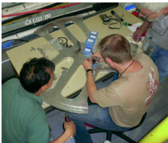
FIG. 1: Vu Thanh Nguyen und Björn Poschen retrieve the graphite crystals from the old chopper wheel. Michael Prager watches closely.
