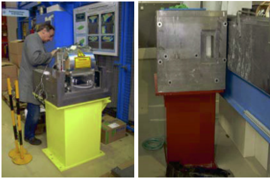
FIG. 2: Left: Last check of the selector shielding. Right: Selector shielding installed in the neutron guide hall at the FRM II.
