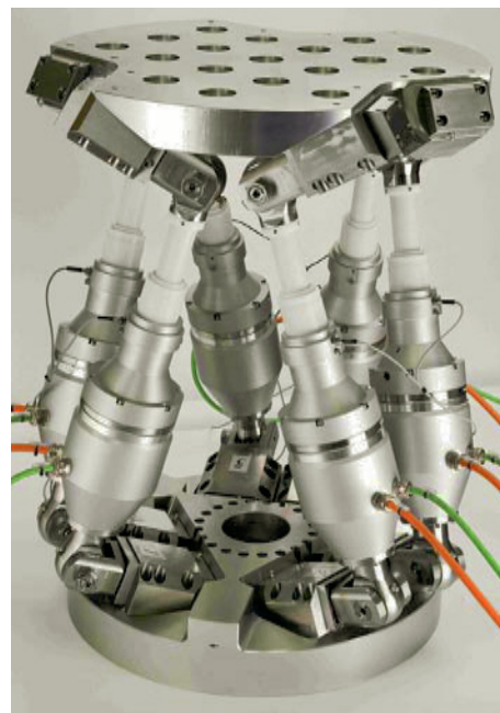
FIG. 5: The Hexapod of the sample table. Below the Hexapod will be an additional turn table and a friction wheel driven detector arm.
