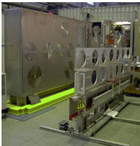
FIG. 3: Polarisation chamber (left) and lifting device (right).
