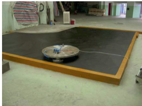
FIG. 5: Dance floor (polished granite floor) around the monochromator shielding area at the SV30 location inside the reactor hall (cf. Fig. 4). The diameter of the mock-up device base plate is 1 m, the load of 1.5 t not shown. The mock-up device is moved on three air pads of exactly the same kind as used with the actual SV30 analyzer/detector tower.
