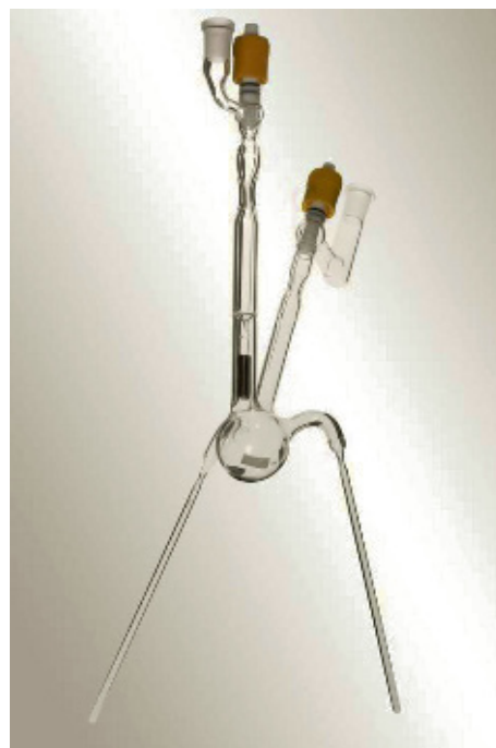
FIG. 1: Reactor for the preparation of NMR samples.
