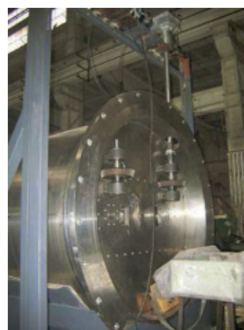
FIG. 2: Twin beam port plug for SV30 at the Chinese reactor CARR before insertion into the respective reactor shielding cavern.
