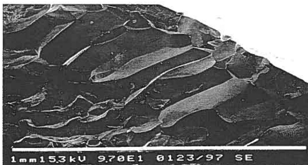
Fig.2: SEM-picture of fused ceramic from BCN18 showing the grain size of about 400 \mu\text{m}
