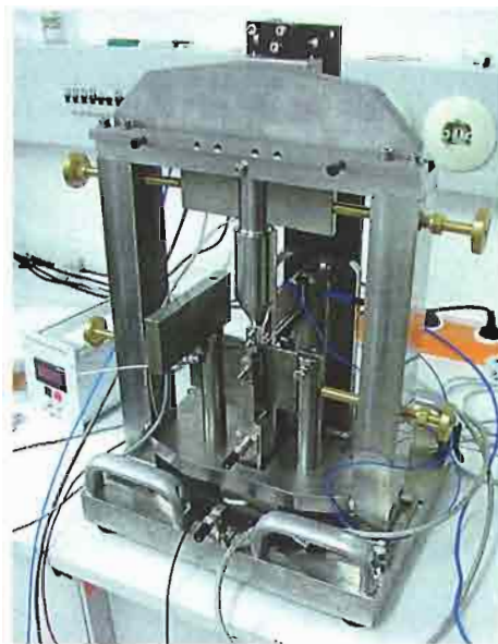
Fig.3 : HCF device for the application of pulsed stresses (FATIMA).
