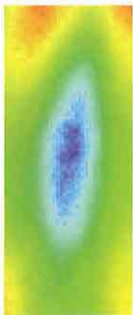
Figure 3. Focus of the PG-monochromator at a neutron energy of 34 meV recorded with a position sensitive detector. The dark blue elliptical area is about 10 mm by 25 mm.
