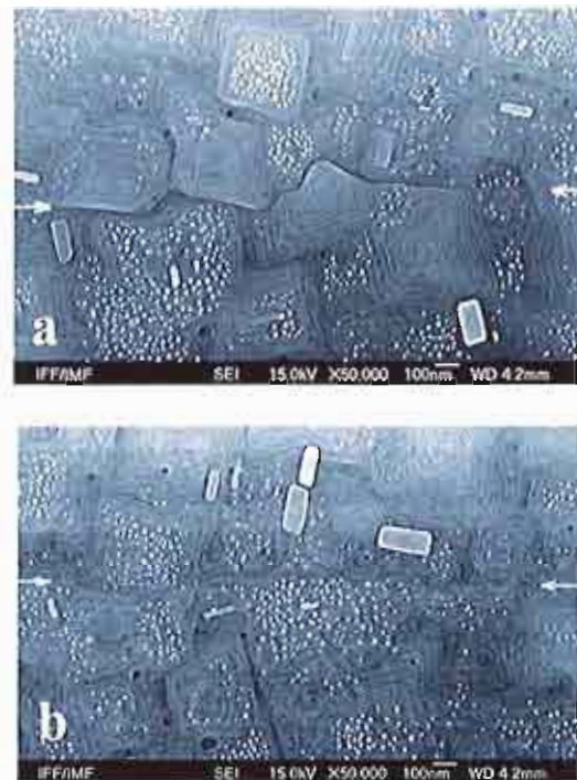
Figure 2 HRSEM images of a bicrystal GB in a YBCO film: (a) GB with a slot and (b) GB without slots.
