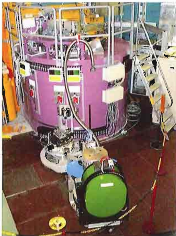
Figure 1. The new spectrometer/diffractometer SV30 at the FRJ-2 reactor. The three beam ports of the monochromator shielding (magenta) can be easily recognized. Sample table and analyzer/detector tower are moved on air cushions across a polished glass floor.
