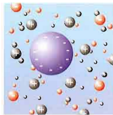
FIG. 1: Sketch of the Primitive Model of charged hard spheres.
