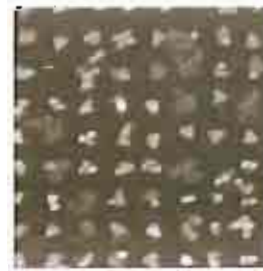
Figure 2: AFM topography scan of a 1 by 1 \mu\text{m}^2 area of lead titanate nanograins. The triangular shape of most grains indicates a (111)-oriented growth induced by the (111) platinum electrode.
