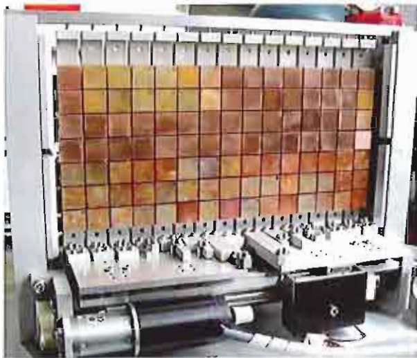
Figure 2. Double-focusing copper monochromator composed of a matrix of 7 by 15 individual single-crystals with an area of 2 \times 2 \text{ cm}^2 each. The columns and rows can be independently rotated in order to enable separate horizontal and vertical focusing.
