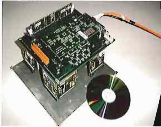
Figure 3. The readout electronics with the FPGA board on the top and edgewise four front end boards with the CIPix-Chip.
