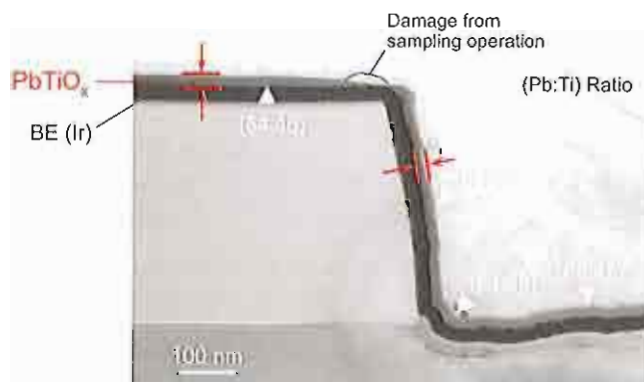
Figure 3: Cross sectional TEM of PbTiO x film deposited on 3D structure pre-covered with Ir bottom electrode layer. The numbers in brackets indicate the local molar ratio of Pb to Ti measured by TEM-EDS. These values were averaged for 3–8 measurements.
