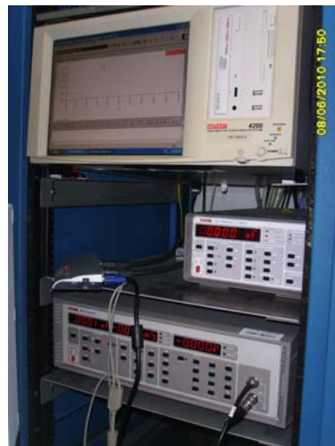
Figure 5. Soft ware interface and the hard ware of Keithley for electric measurement. From above to bottom is Keithley interface test environment, Keithley 595 Quasistatic CV meter, Keithley 590 CV analyzer respectively.
