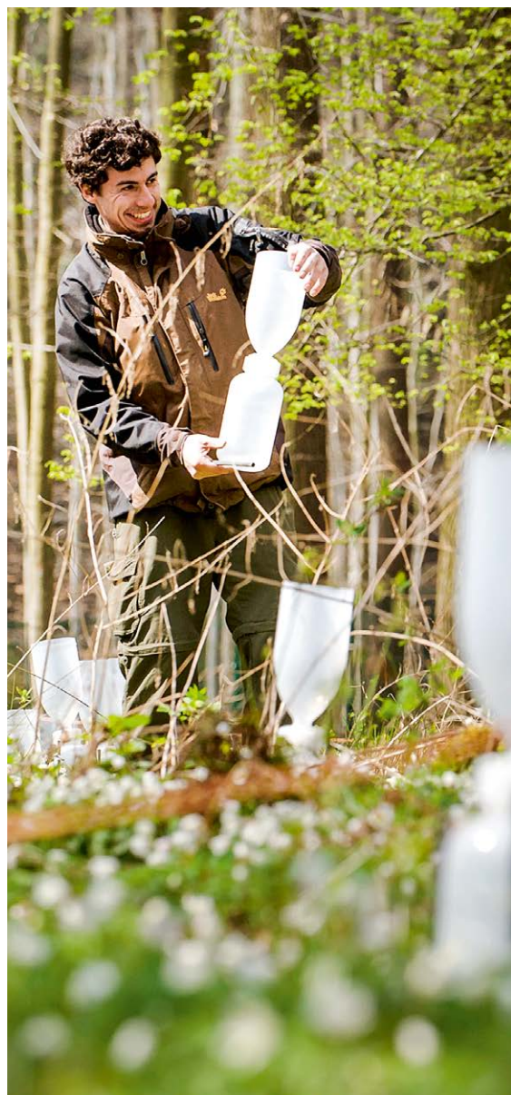
Distributing and installing rain collectors in a mixed beech forest
