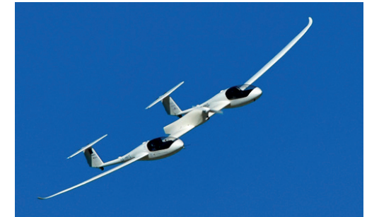
HY4 – first four-seater passenger aircraft powered solely by a hydrogen fuel cell battery system (DLR)
