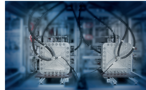
Polymer electrolyte membrane-based stack combination used for characterization in electrolysis test stand (FZJ)
