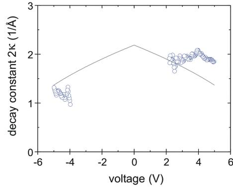
FIG. 3: Decay constant  $2\kappa$  as a function of the voltage (open circles). The solid line shows the calculated trend for tunneling with zero parallel wave vector. These data reflect the dispersion of the surface states.
