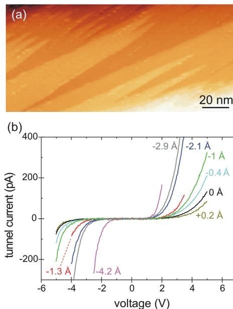
FIG. 1: (a) Constant-current empty state STM image of a cleaved GaN( $1\bar{1}00$ ) surface. (b) Current-voltage spectra measured on the flat terraces. The different curves correspond to different tip-sample separations  $z = z_0 + \Delta z$  ( $\Delta z$  given at each curve and  $z_0$  defined by a set voltage and current).
