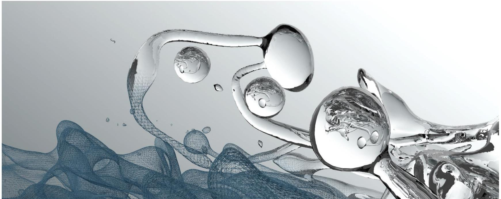
rendered with Blender from a DNS of a diesel injection spray of ITV, RWTH Aachen University
