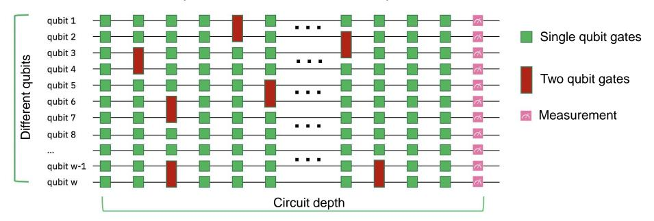
A quantum circuit of width w and depth d
