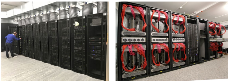
Large-scale SpiNNaker and BrainScaleS systems at the University of Manchester and Heidelberg University
