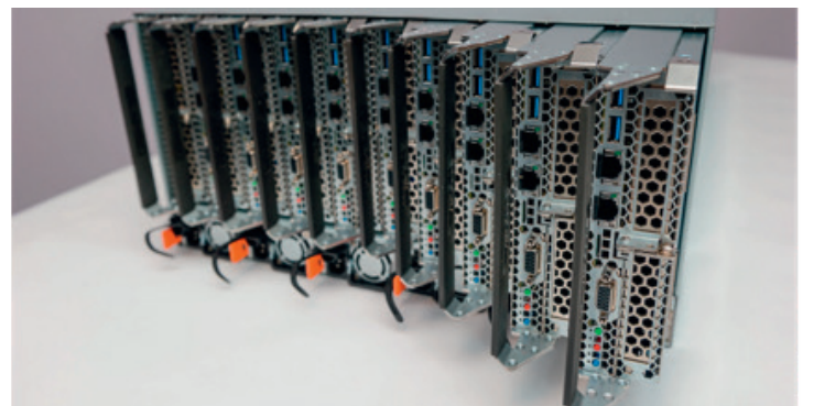
View of the T-Platforms V5050 chassis. Each chassis can host ten V210S or, alternatively, five GPU-equipped V210F blades.
