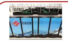
**Piz Daint XC50 @ CSCS:** Model: Xeon E5-2690 v3 (HSW) @ 2.60 GHz Cores: 1x12 = 12 Accelerators: 1 x P100 RAM: 64 GB/node
