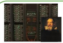
Galileo @ CINECA Model: Xeon E5-2630 v3 (HSW) @ 2.40 GHz Cores: 2x8 = 16 Accelerators: 2 x K80 RAM: 128 GB/node
