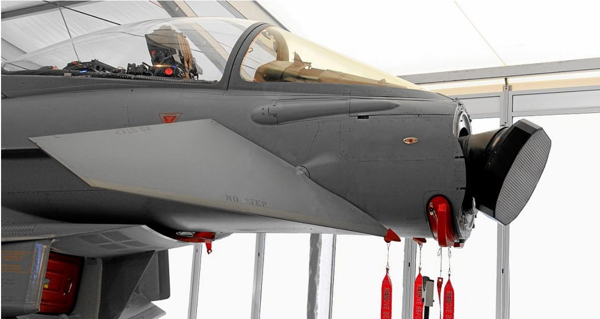
CAPTOR-E active phased-array radar in the nose of a Eurofighter Typhoon
