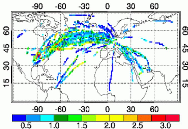
*Climatology of NO<sub>y</sub> in the upper troposphere ( $z > 8\text{km}$ ,  $O_3 < 100\text{ppb}$ ) compiled from the MOZAIC-data between April '01 and Feb '02. The color scale gives the mixing ratio in ppb ( $10^{-9}$ ). The individual measurements were averaged on a  $1^\circ \times 1^\circ$  grid.*
