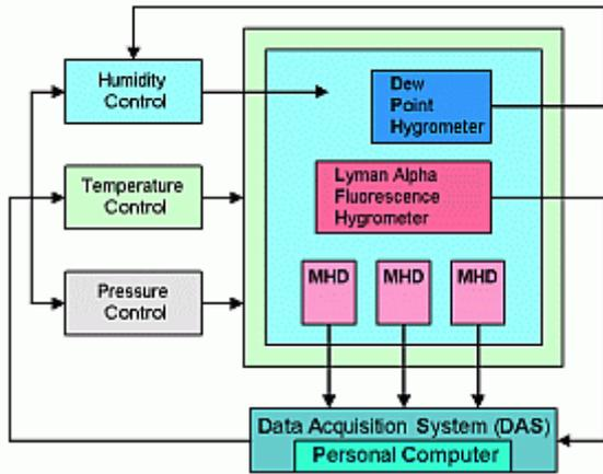
**Figure 3:** Scheme of the set up for the calibration of humidity sensing devices in the environmental simulation chamber
