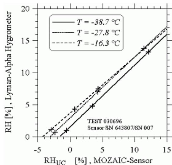
**Figure 6:** The calibration of a MOZAIC humidity sensor in the environmental simulation chamber results in three linear calibration curves at three different temperatures.
