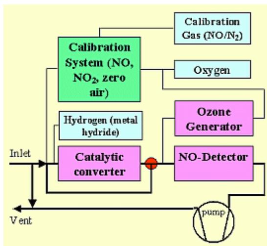
Principle of the NO<sub>y</sub>-Instrument.
