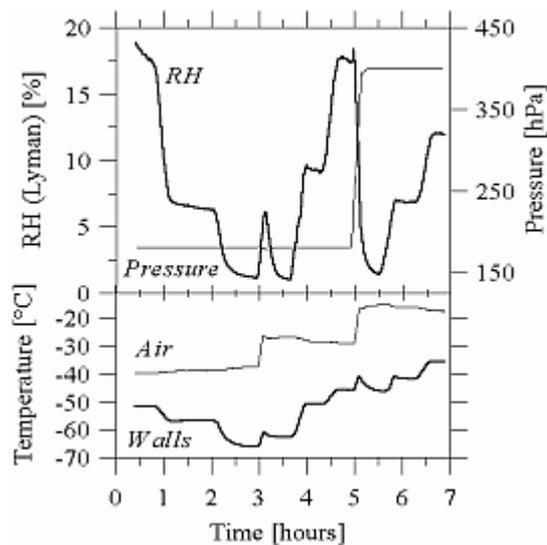
**Figure 5:** Water vapor calibration run in the environmental simulation chamber as function of simulation time. Shown are RH, measured by Lyman-Alpha fluorescence hygrometer, pressure, air temperature, and temperature of the chamber walls.
