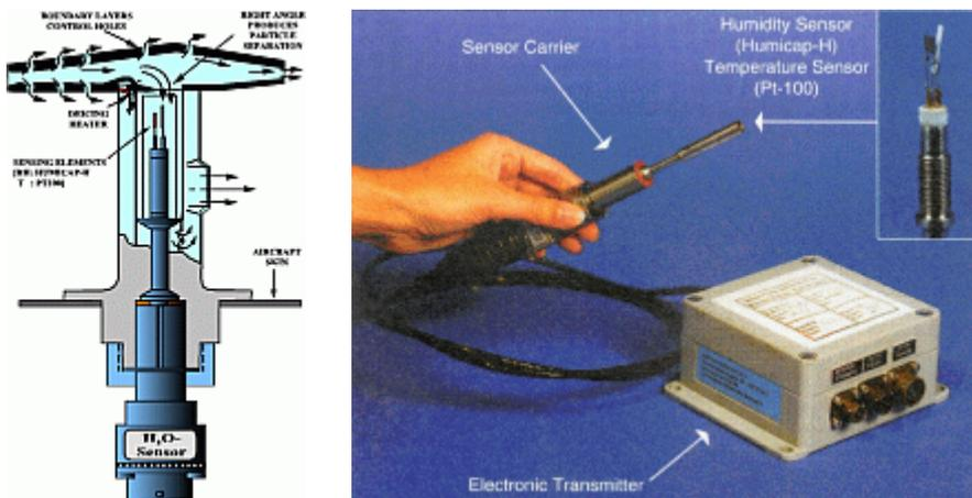
**Figure 2:** Left panel: Cross section of the airborne MOZAIC humidity sensor mounted in air sampling housing (Rosemount, Model 102 BX). Right panel: MOZAIC Humidity Device (MHD) to be installed in a Rosemount housing mounted on the outside skin of the Airbus A340 aircraft (see Figure 1).
