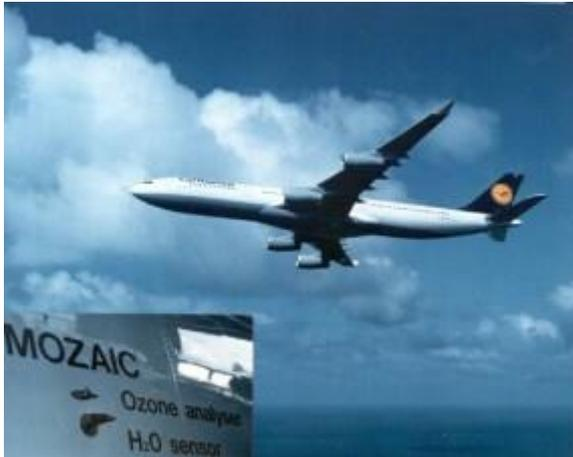
**Figure 1:** Airbus A340 equipped with MOZAIC-Humidity Device. Inlet system mounted at the outside skin of the aircraft close to the cone.
