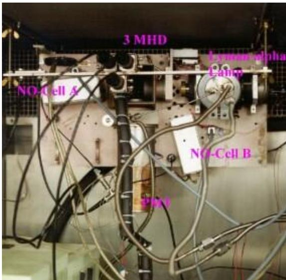
**Figure 4:** Three MOZAIC-Humidity Devices (MHD) installed at the outlet of the air sampling duct of the Lyman ( $\alpha$ ) Fluorescence Hygrometer (LFH) in the environmental simulation chamber just prior to a calibration run.
