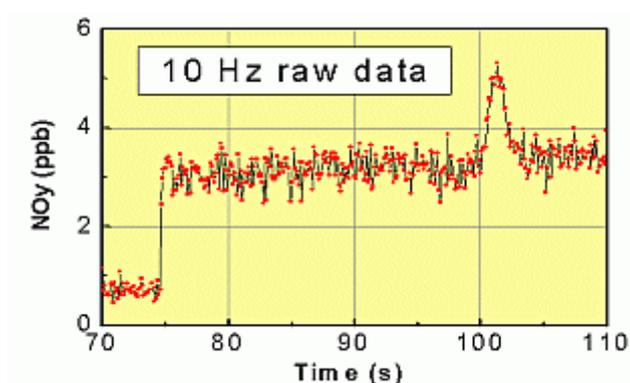
The high time resolution of 0.1 s (corresponding to a distance of 30 m at cruise level) allows to identify aircraft emissions and other recent sources in the raw data.
