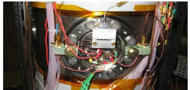
Fig. 46: Cs apparatus mounted on a Ioffe trap with feed-throughs for photodiodes, Stark shifting plates, field ionization plates, getter current, and temperature sensor. The optical fiber at the top carries both excitation wavelengths.
